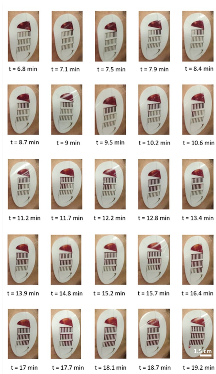
Fig. S4. Calculation of sweat rate using the wearable Cap -Drop-Sweat system containing 24 CHs.
