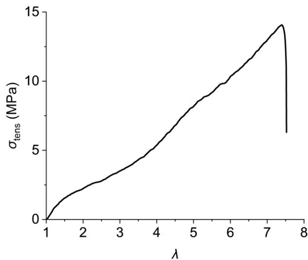
Figure S2. Tensile testing of free-standing polyurethane.
