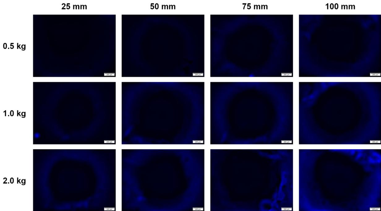
Figure S5. Fluorescence microscopic images of the impact areas of the clear coating that was struck by a falling punch of different weights (left) and from different heights.
