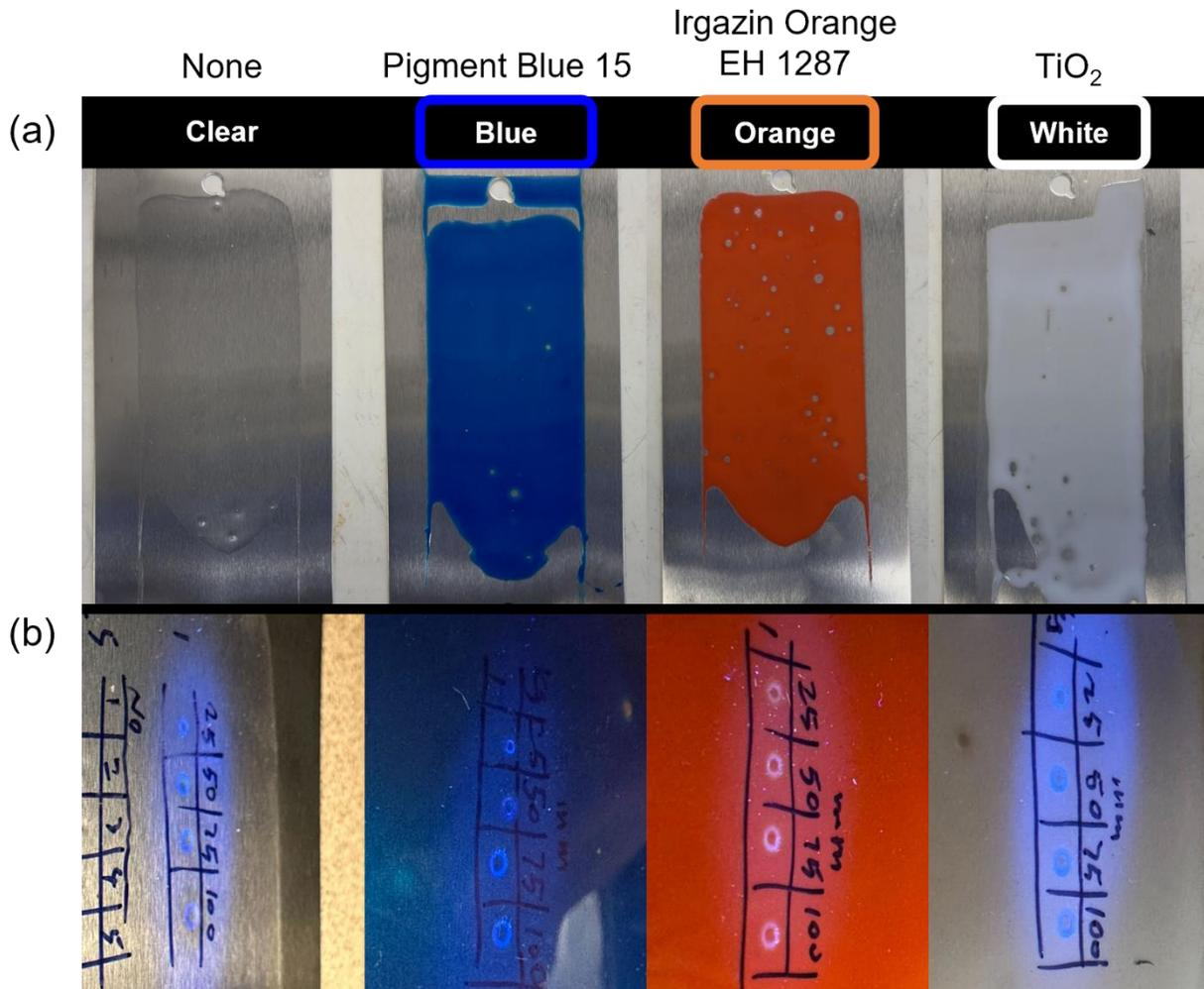
Figure S8. (a) Photos of the clear and pigmented coatings on steel substrate. (b) Photos of the coatings after impact by a punch of 1.0 kg falling from different heights as indicated by the numbers above the spots of impact, on which the mechanically generated fluorescence was visualized under a UV flashlight ( $\lambda_{\text{max}} = 365 \text{ nm}$ ).
