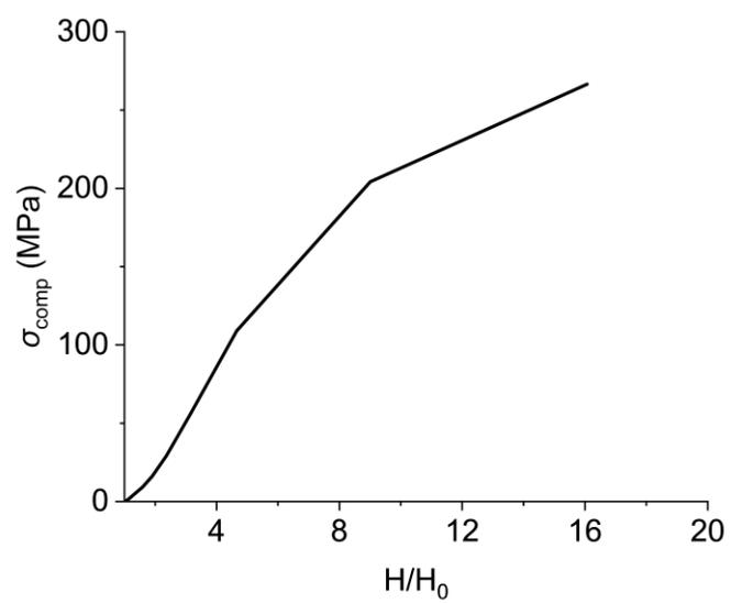
Figure S3. Compressive testing of free-standing polyurethane.
