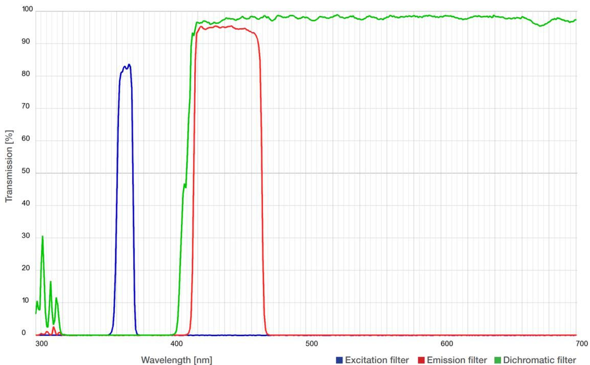
Figure S7. Transmission of the U-FUNA Fluorescence Filter Cube (from manufacturer [https://www.olympus-lifescience.com/en/optics/mirror-units/#!cms\[focus\]=cmsContent6353](https://www.olympus-lifescience.com/en/optics/mirror-units/#!cms[focus]=cmsContent6353)).
