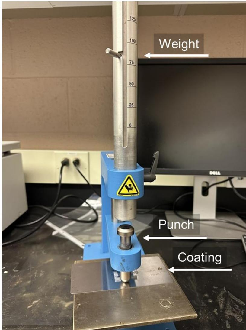
Figure S4. Setup for the impact experiments.
