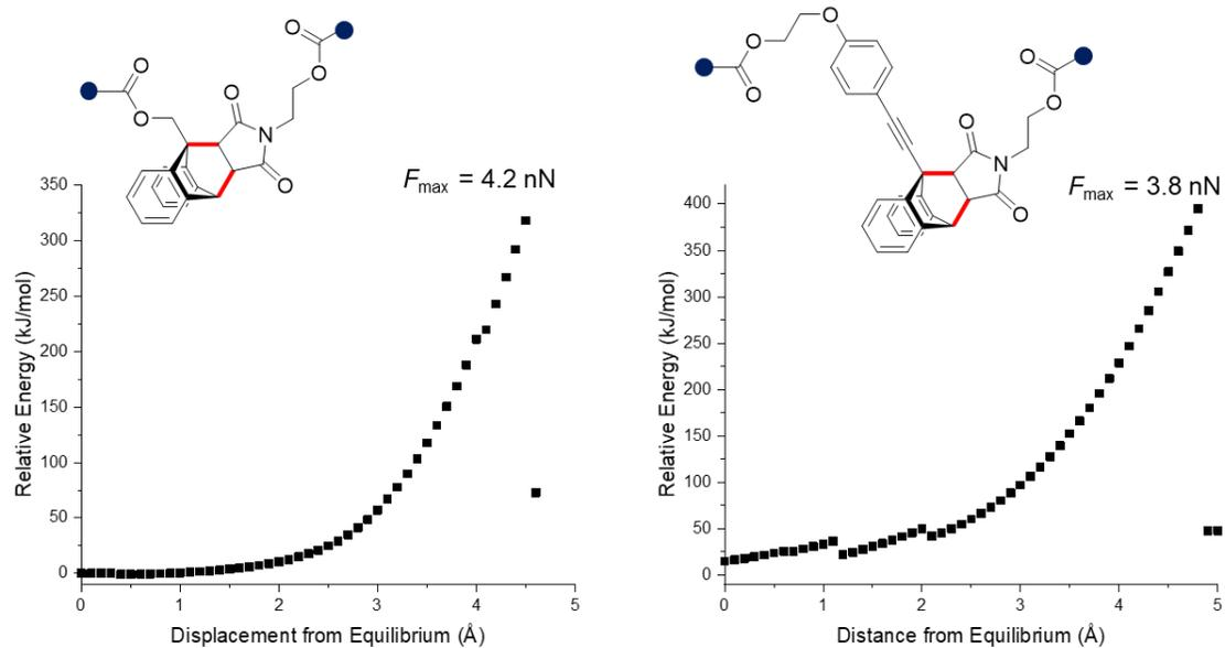
Figure S1. Constrained geometries simulate external force (CoGEF) calculation results for anthracene-maleimide (left) and  $\pi$ -extended anthracene-maleimide (right) cycloadducts.
