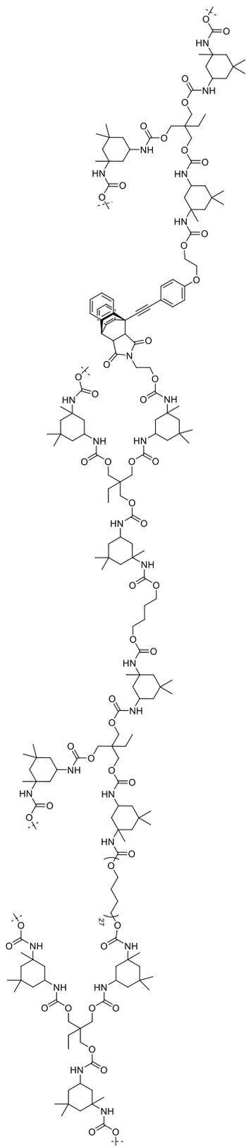
Figure 11. Structure of the PU network.
