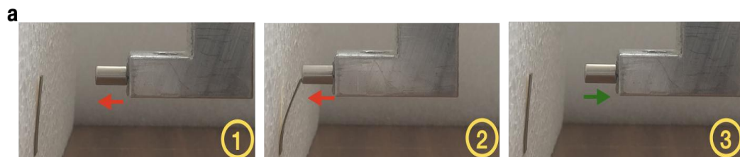
Fig. S6 Deformation of the mTPU/Au bi-layer upon the approach and withdrawal of a permanent magnet.
