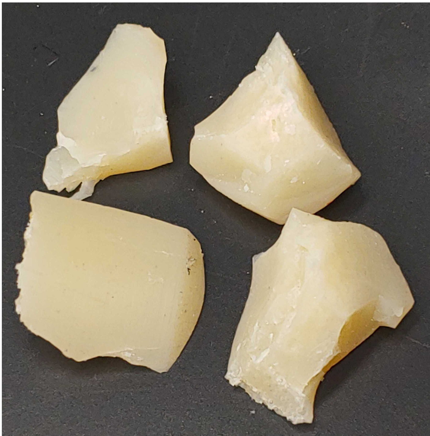
Fig. S7 Visual results of the PA6-MULCH-10. The glossy sheen and the white color are indicative of a high molecular weight polymer with no oxidation occurring during polymerization. The molecular weight was corroborated with GPC and demonstrated the effective polymerization
