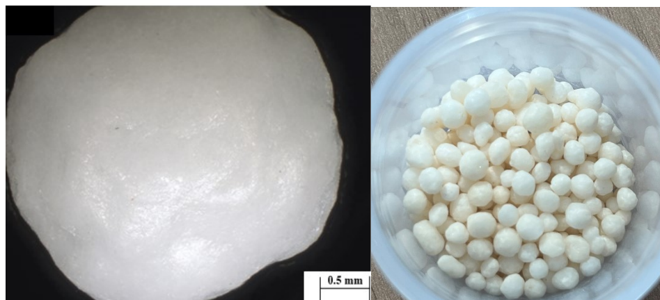
Figure S2. (Left) Magnified microscope picture of urea (46-0-0) coated with 2.7 wt% PU and 0.5 wt% wax additive. (Right) Picture of coated urea (46-0-0) batch.
