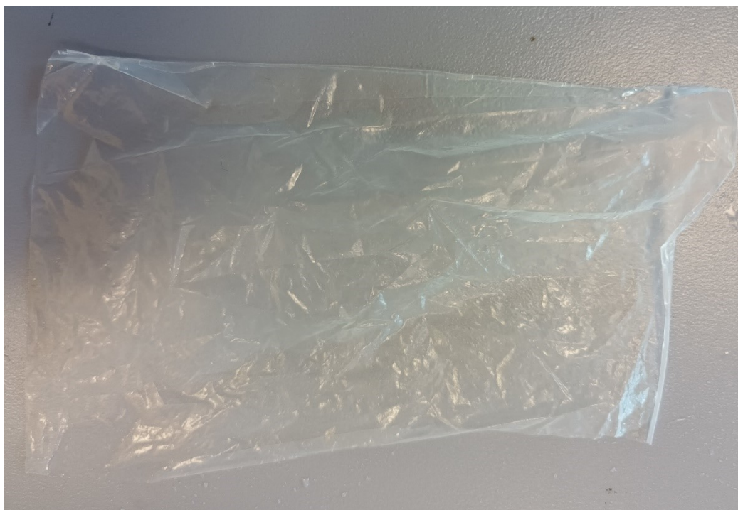
Figure S4 Photo of a typical RG-AEM. No obvious structural defects are observed on the macroscale.
