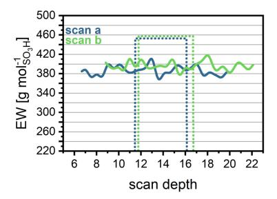
d) Mean EW vs membrane depth and reinforcement position vs membrane depth-averaged over all S390 (BOL) samples.
