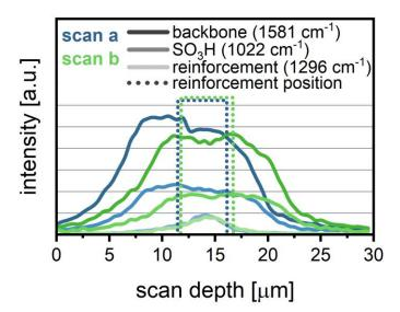
c) Two exemplary EW-depth-scan for reinforced S390 (BOL; same scans as in b): Solid lines are the EW depending on absolute scan depth for all areas where the membrane is detected. Dotted lines: scan-depth where reinforcement is detected (50% of max intensity for the signal at 1296 cm<sup>-1</sup>).
