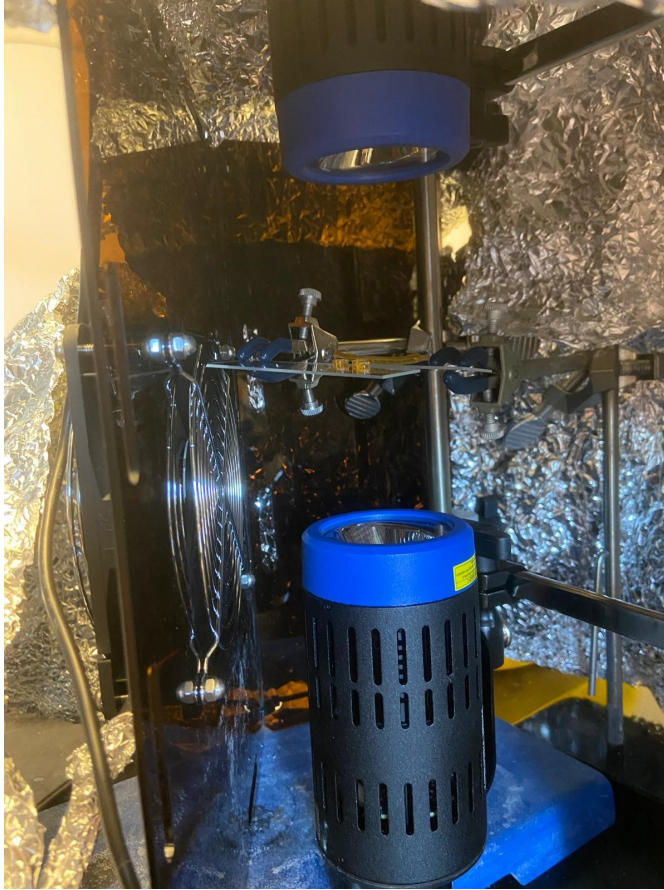
Figure S3. PETG material held between two UV lamps
