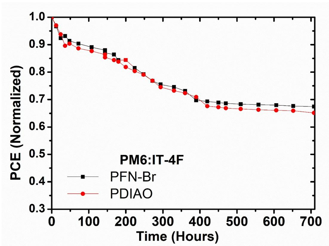
**Figure S6.** Stability studies of PM6:IT-4F based OPV devices with PFN-br and PDAIO interlayer. All devices are stored in a glove box between the J-V measurements.
