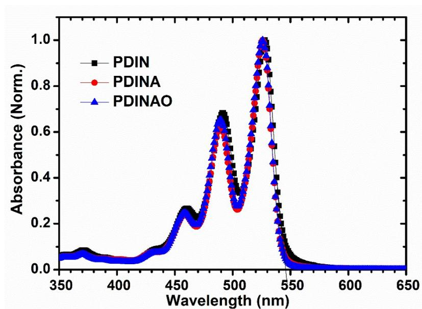
Figure S2. Optical absorption spectra of PDIN, PDIA and PDIAO in solution form.
