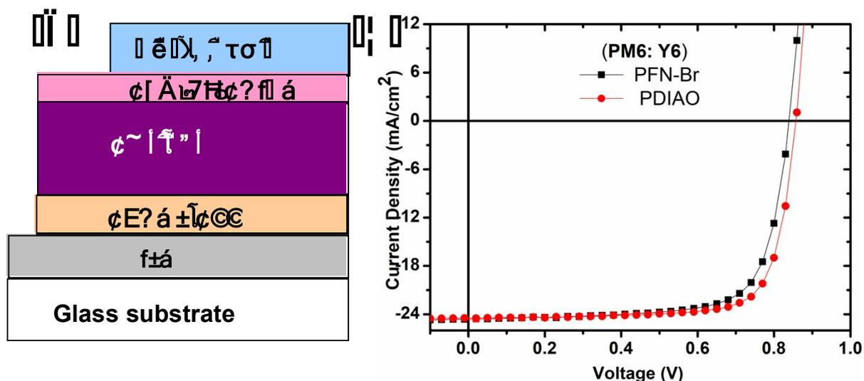
**Figure S4.** A. Schematic diagram of OPV device and (b) J-V plot of PM6:Y6-based OPV devices with PFN-Br and PDIAO ETL materials.
