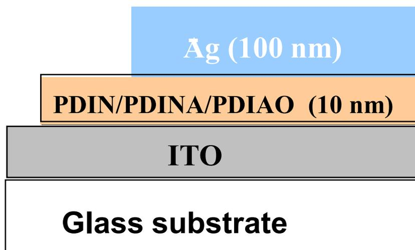
**Figure S5.** Schematic diagram of a device used for conductivity studies.
