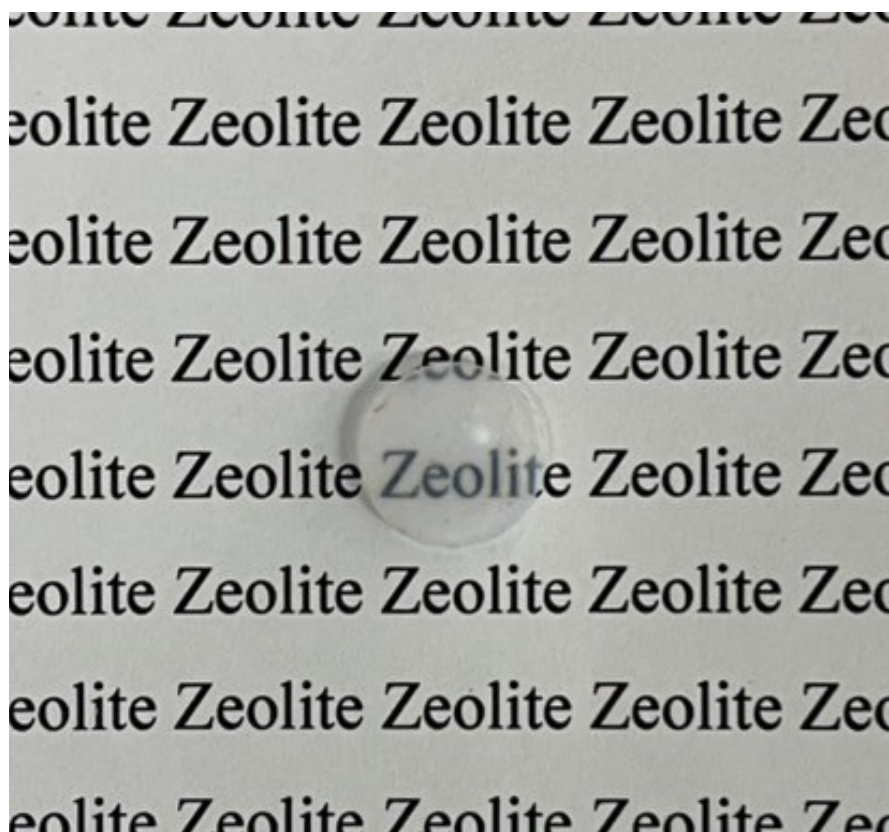
Figure S2. Photograph of silicalite-1 ceramic corresponding to the one shown in Figure 1(a) after a drop of water was applied.
