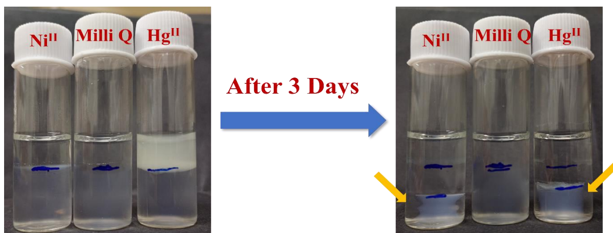
Fig. S5 A control syneresis study of Fmoc- 1 Nap-A hydrogel in the presence of Ni II ions, milli Q water and Hg II ions solutions.
