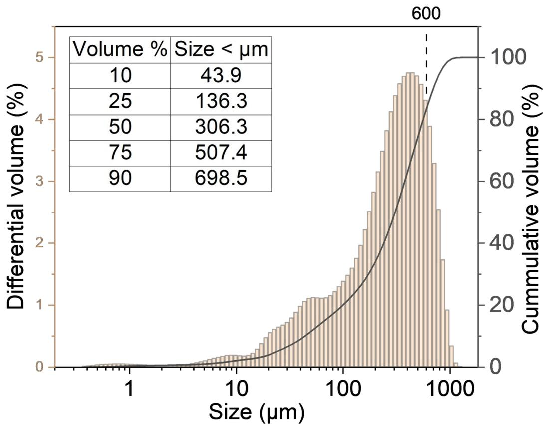
*Fig. S4 Particle size distribution of the rapeseed straw powder. The milled rapeseed has a mean size of 342.5  $\mu\text{m}$  and a median size of 306.3  $\mu\text{m}$ .*
