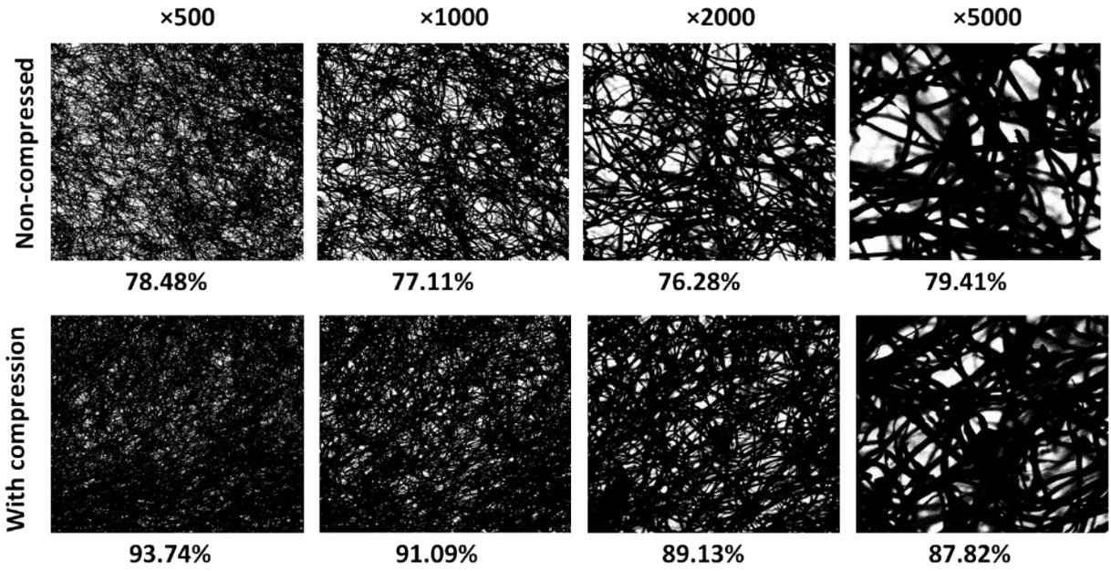
*Fig. S3 A densification of hyphal network can be observed after compression. Hyphal projected density calculated after adjusting the threshold of SEM images at ×500, ×1000, ×2000, and ×5000 magnifications.*
