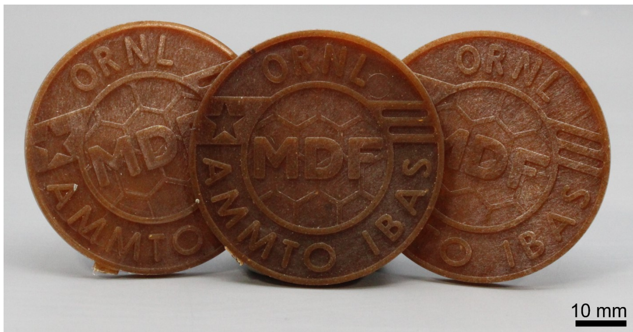
Figure S9. A coin was injection molded from the scaled composite seen in Figure S8 , to demonstrate the ability of this material to be injection molded. In this case, an APSX-PIM V3 Plastic Injection Machine was used to injection mold these materials at a temperature of 190 °C, an injection pressure of 220 bar, a hold pressure of 18 bar, and a hold time of 6 seconds.
