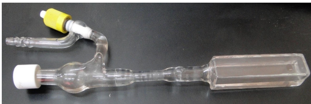
Fig.S.9. The experiments have been conducted in the above photocatalytic reactor.
