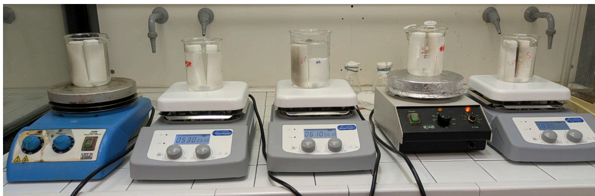
Figure S20: Experimental set-up for the acid attack resistance test.
