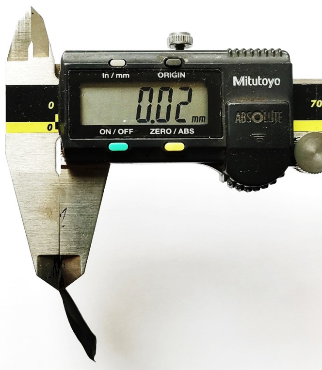
Fig. S1: Digital photograph showing thickness of flexible SM substrate.
