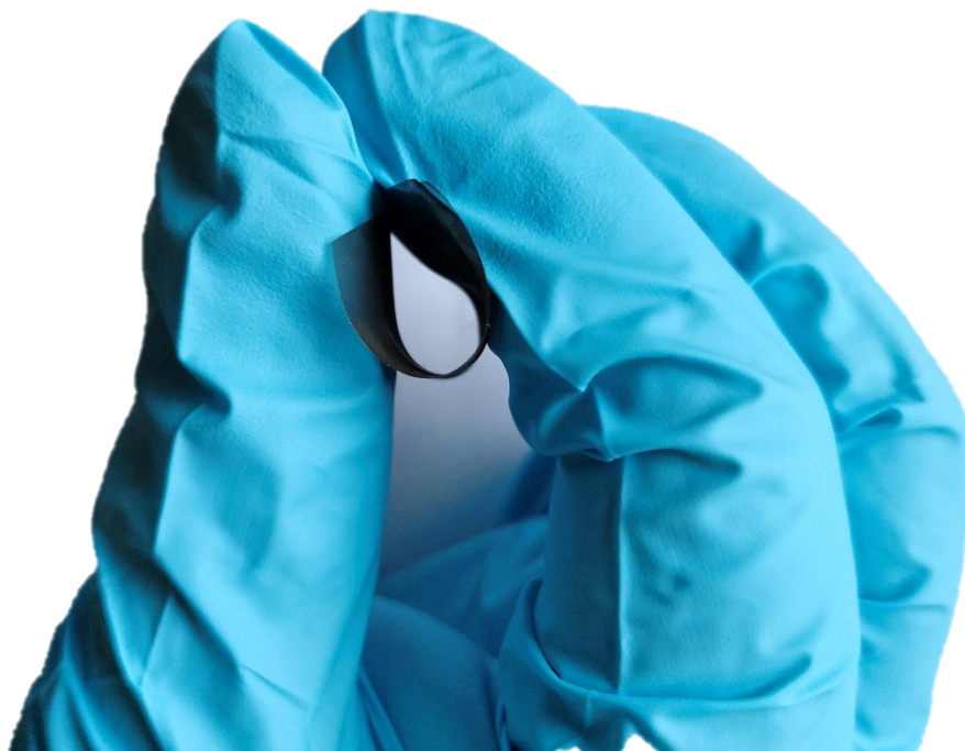
Fig. S2: Digital photograph showing flexibility of the electrode.
