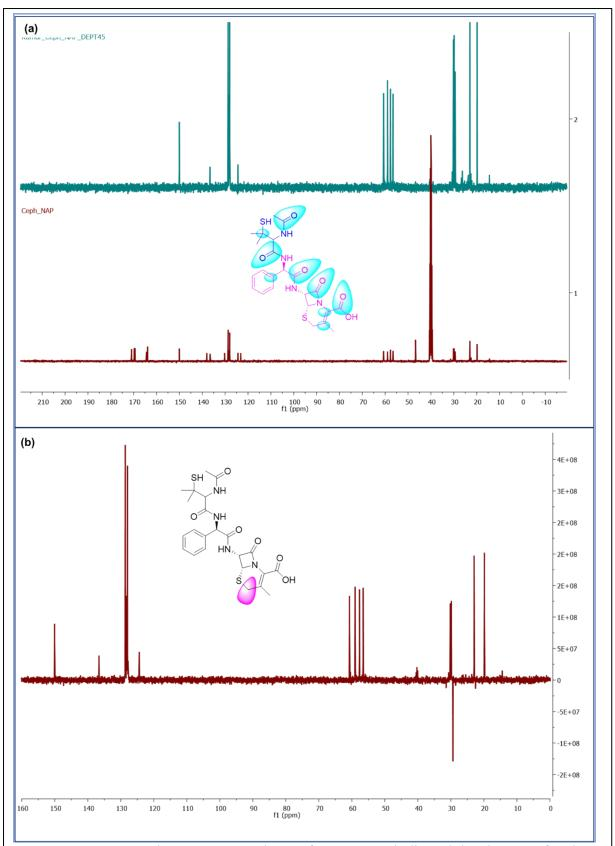
**Fig. S7**. DEPT\_45 and DEPT\_135 analyses of NAP\_CEX indicated the absence of carbons without attached protons (7**a**) and the presence of a single CH<sub>2</sub> group (7**b**).
