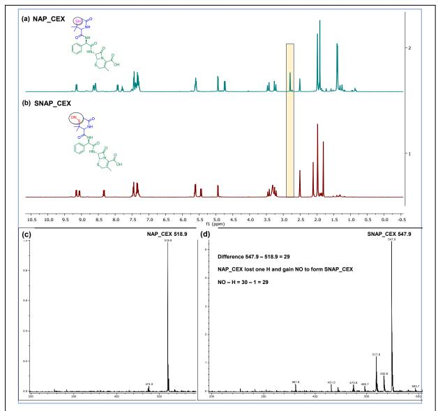
**Fig. S8.** (a-b) Characterization of the conversion of thiol to nitroso group in the target compound: Proton NMR comparison for NAP\_CEX (1a) and SNAP\_CEX (1b). (c-d) ESI-Mass analysis indicates the clear conversion of NAP\_CEX (1b) to SNAP\_CEX (1d).
