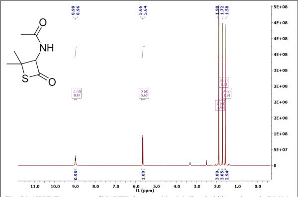
**Fig. S1**. 1H NMR spectrum of NAPTH; 3-acetamido-4,4-dimethylthietan-2-one in DMSO-d<sub>6</sub>.
