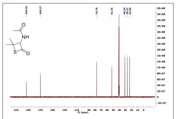
**Fig. S2**. 13C NMR spectrum of NAPTH; 3-acetamido-4,4-dimethylthietan-2-one in DMSO-d<sub>6</sub>.
