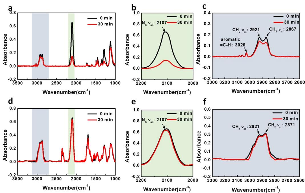
**Figure S7** FTIR spectra of homopolymer and azide blend films before and after UV light exposure: (a) PS and azide blend film with enlarged region ranged from (b) 2200  $\text{cm}^{-1}$  to 2000  $\text{cm}^{-1}$  and (c) 3300  $\text{cm}^{-1}$  to 2600  $\text{cm}^{-1}$ ; (d) PMAA and azide blend film with enlarged region ranged from (e) 2200  $\text{cm}^{-1}$  to 2000  $\text{cm}^{-1}$  and (f) 3300  $\text{cm}^{-1}$  to 2600  $\text{cm}^{-1}$ .
