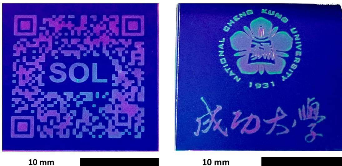
**Figure S4.** Photo-patterned DPP-DTT film with millimeter-scale dimension.
