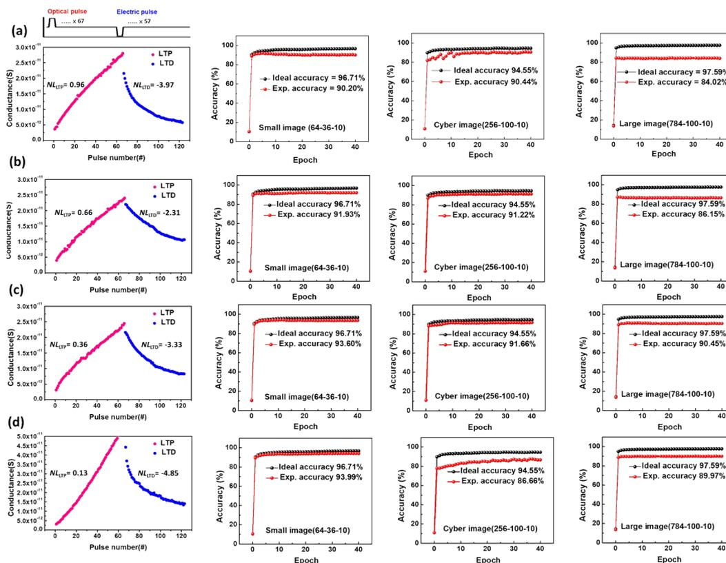
**Figure S11.** Four cycles of repeated LTP and LTD response by optical and electric pulse trains and the corresponding accuracy. (a) first cycle, (b) second cycle, (c) third cycle and (d) fourth cycle.
