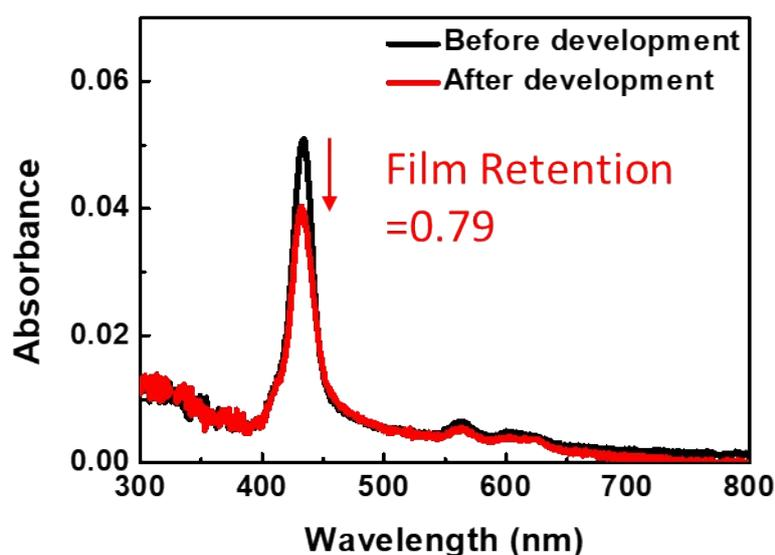
**Figure S8.** Absorption spectra of photo-crosslinked BCP/ZnTPP before and after development.
