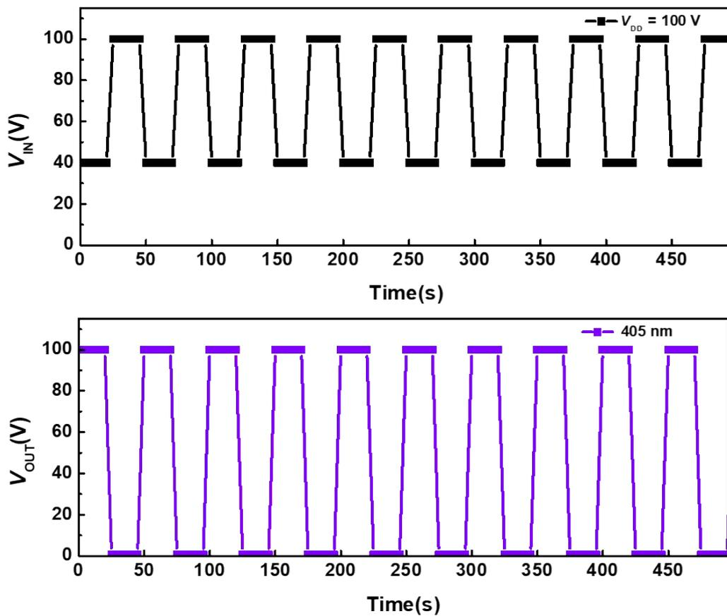
**Figure S13.** Time traces of the input and output voltage for inverter consisting of DPP-DTT based OFET and BCP/N2200 based OFET under 405 nm light illumination.
