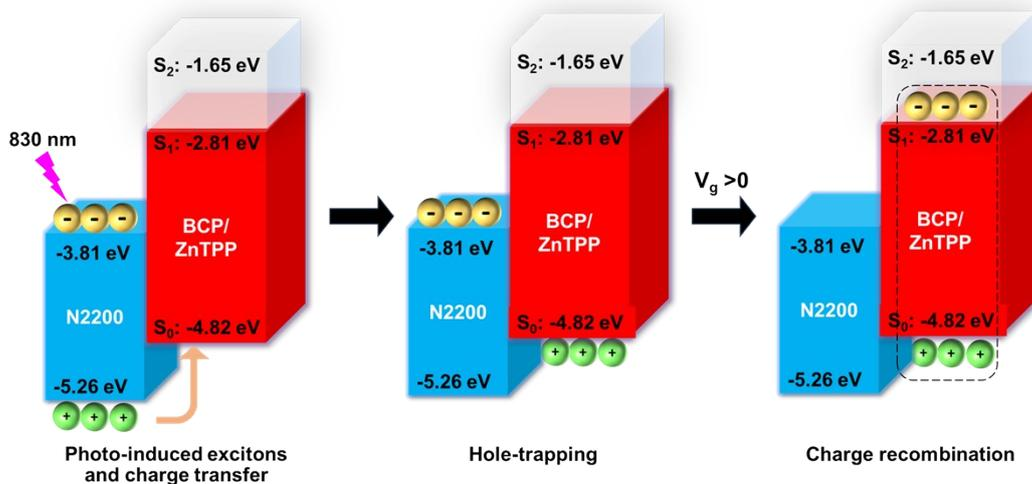
**Figure S10.** The proposed mechanism of photo-recordable behavior by lower photon energy.
