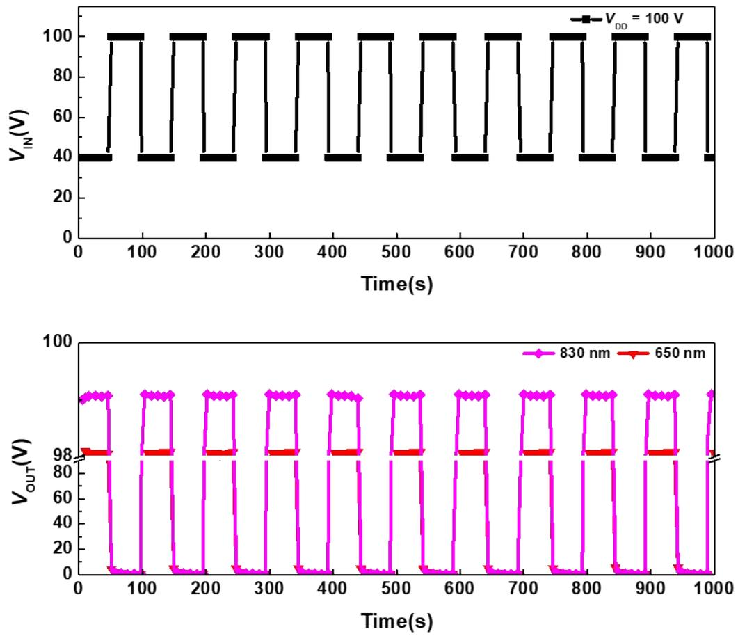
**Figure S12.** Switching characteristics of the photo-programmable inverter under 830 nm and 650 nm light stimuli.
