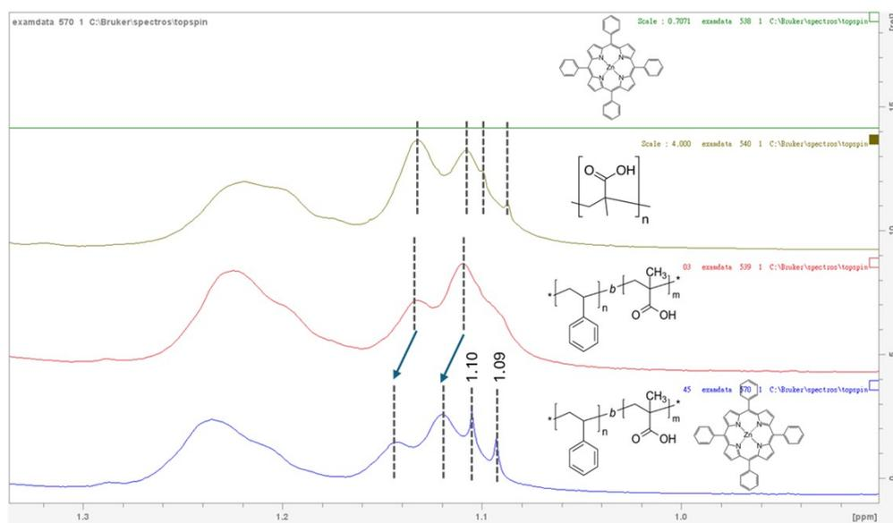
**Figure S2.** Solution  $^1\text{H}$  NMR spectra of (a) ZnTPP, PMAA, PS-*b*-PMAA and PS-*b*-PMAA/ZnTPP, (b) ZnTPP, (c) PMAA, (d) PS-*b*-PMAA and (e) PS-*b*-PMAA/ZnTPP. (f) ZnTPP, PMAA, PS-*b*-PMAA and PS-*b*-PMAA/ZnTPP with the spectra ranged from 1.35 ppm to 0.99 ppm.
