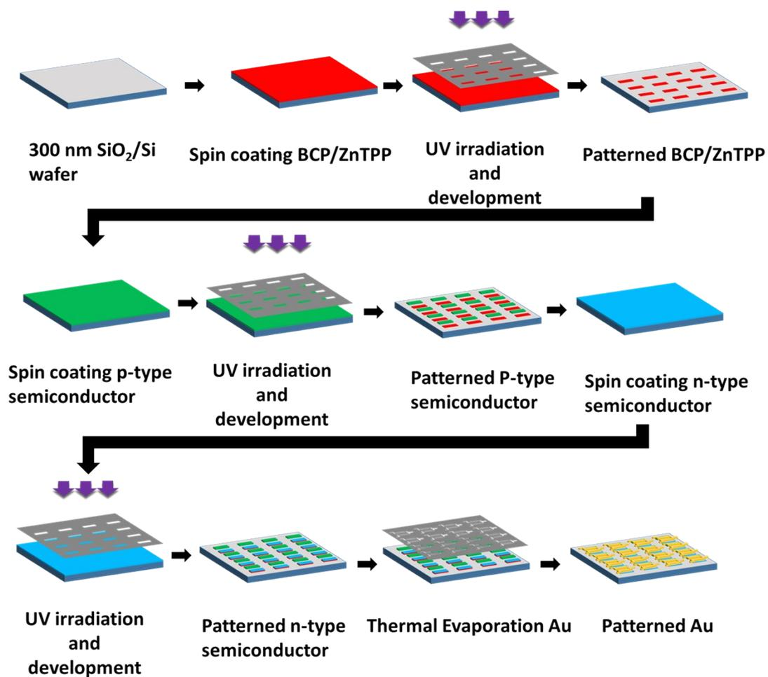
**Figure S1.** Schematic description of the fabrication processes for photopatterned and photo-programmable logic gate through photopatterning using azide as photo-crosslinker.
