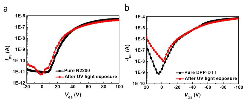
**Figure S5.** Stability test of conjugated polymer under UV light exposure. Transfer curves of (a) pure N2200 derived FET and (b) pure DPP-DTT derived FET.
