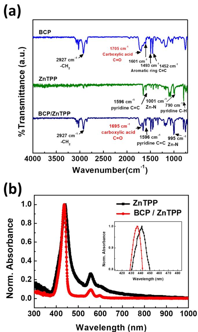
**Figure S3.** (a) FTIR spectra of BCP, ZnTPP and BCP/ZnTPP film to confirm the chelating effect between BCP and ZnTPP. (b) The absorption spectra of ZnTPP and BCP/ZnTPP film.
