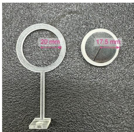
**Fig. S4.** 3D printed ring-shaped structures for blocking the objects'  $x$ - $y$  plane movement.
