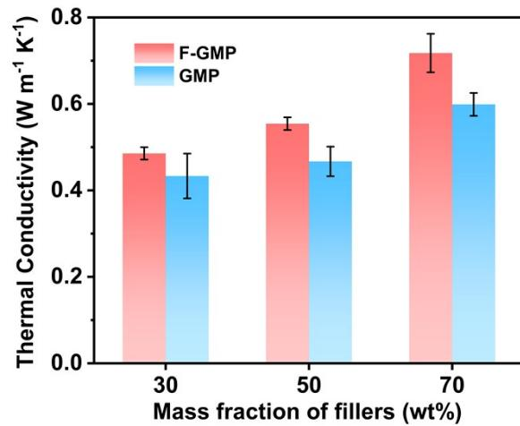
**Figure S17.** Through-plane thermal conductivity of the composite films.
