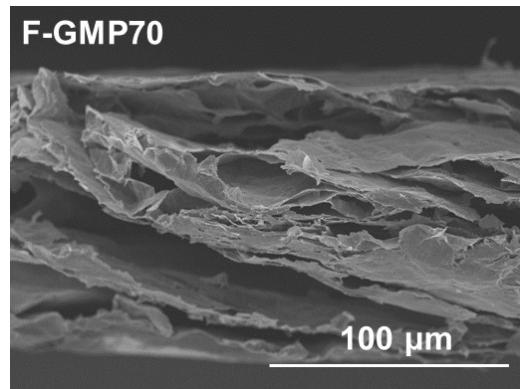
**Figure S10.** Cross-sectional SEM image of the F-GMP70 composite film.
