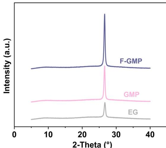
**Figure S7.** XRD patterns of pristine EG, F-GMP, and GMP.
