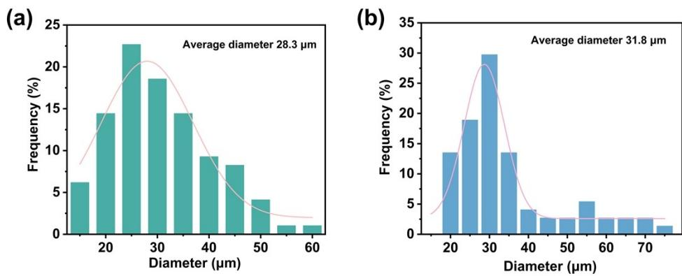
**Figure S16.** Dimensional statistics of (a) F-GMP and (b) GMP.
