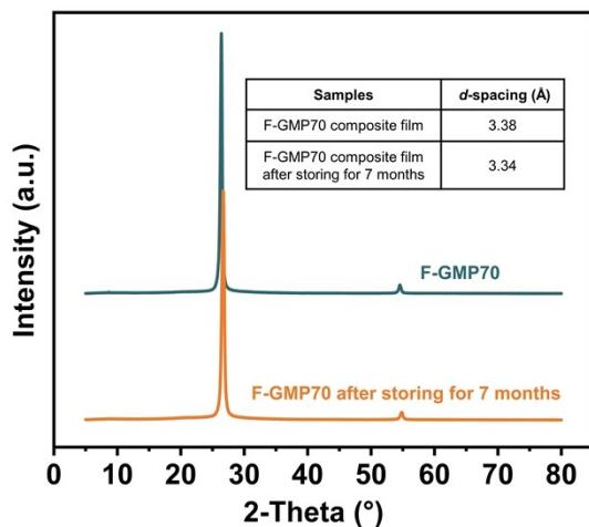
**Figure S20.** XRD patterns of the F-GMP70 composite film before and after storing for 7 months.
