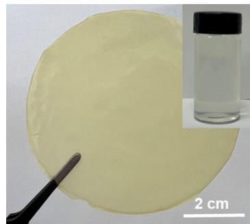
**Figure S1.** Digital photos of the ANF film and the ANF/DMSO/DI dispersion.
