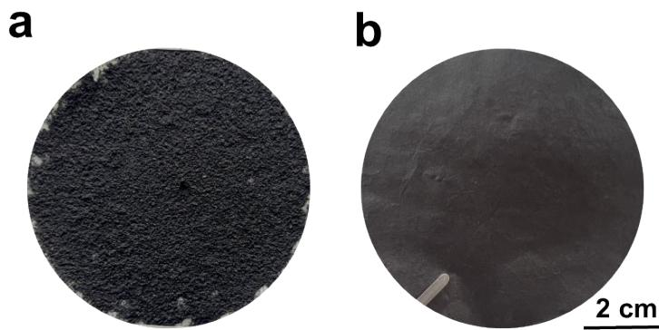
**Figure S19.** Digital photos of the composite films prepared from (a) GMP/ANF and (b) F-GMP/ANF pastes after the long-term storage for 7 days.
