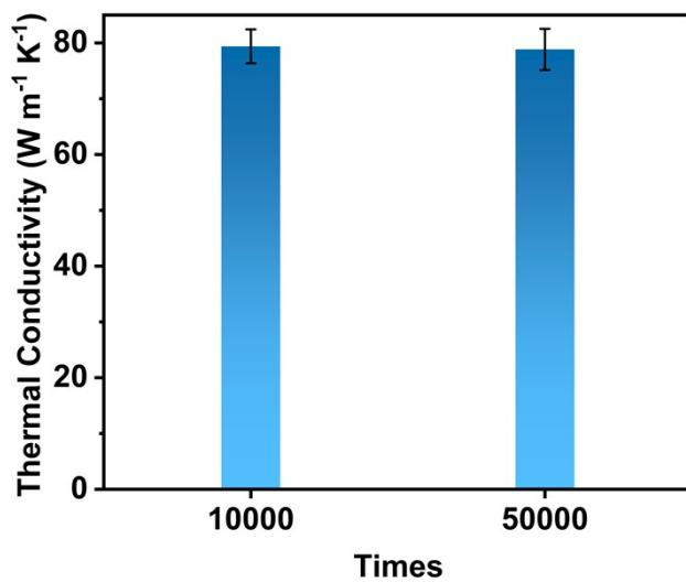
**Figure S15.** Thermal conductivity variation of the F-GMP70 composite film after bending for 10,000 and 50,000 times.
