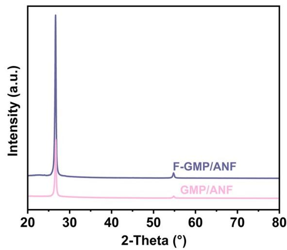
**Figure S12.** XRD patterns of the F-GMP/ANF and GMP/ANF composite films.
