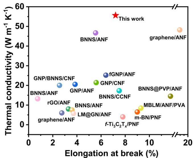
**Figure S14.** A comparison of the thermal conductivity and the elongation at break between the composite films developed in this work and previously-reported nanofiber-based thermally conductive composite films [S1-16].
