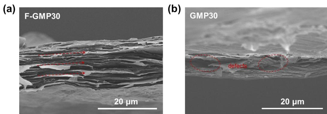
**Figure S8.** Cross-sectional SEM images of the (a) F-GMP30 and (b) GMP30 composite films.
