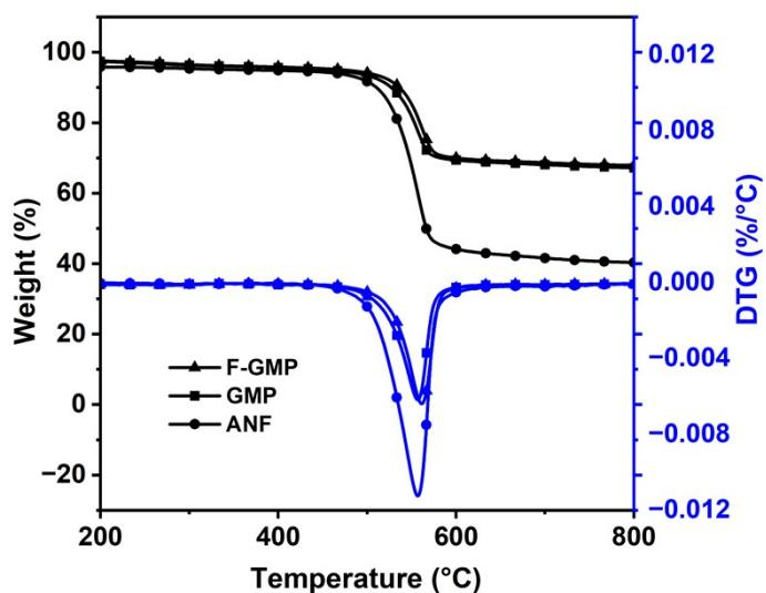
**Figure S9.** TGA and DTG curves of ANF, F-GMP and GMP composite films.
