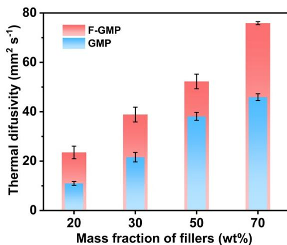
**Figure S11.** In-plane thermal diffusivity of the composite films.
