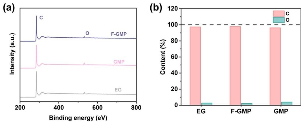
**Figure S6.** (a) XPS spectra of pristine EG, F-GMP, and GMP. (b) Oxygen and carbon contents in EG, F-GMP, and GMP.
