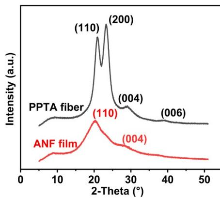
**Figure S2.** XRD patterns of pristine PPTA fiber and ANF film.
