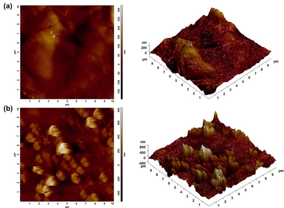
**Figure S13.** AFM images of (a) F-GMP/ANF and (b) GMP/ANF composite films.
