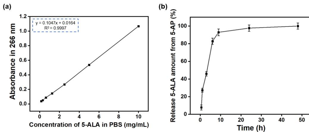
**Fig. S1.** (a) UV/vis absorption-based standard curve of 5-ALA to analyze the release efficiency of 5-AP. (b) Release profile of the 5-ALA from 5-AP. The data are presented as means  $\pm$  S.E.M. (n = 3).
