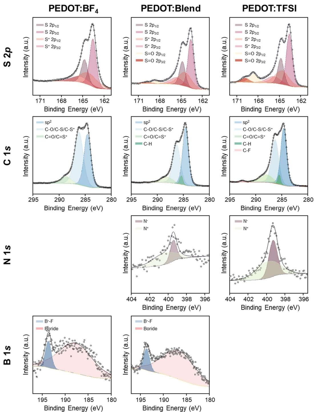
**Figure S6.** S 2p, C 1s, N 1s and B 1s XPS spectra of PEDOT: BF<sub>4</sub>, PEDOT:Blend, and PEDOT:TFSI thin films.
