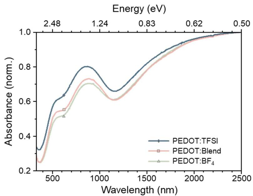
**Fig. S7** Normalized UV-Vis-NIR absorbance spectra of the three OSIEPed films.
