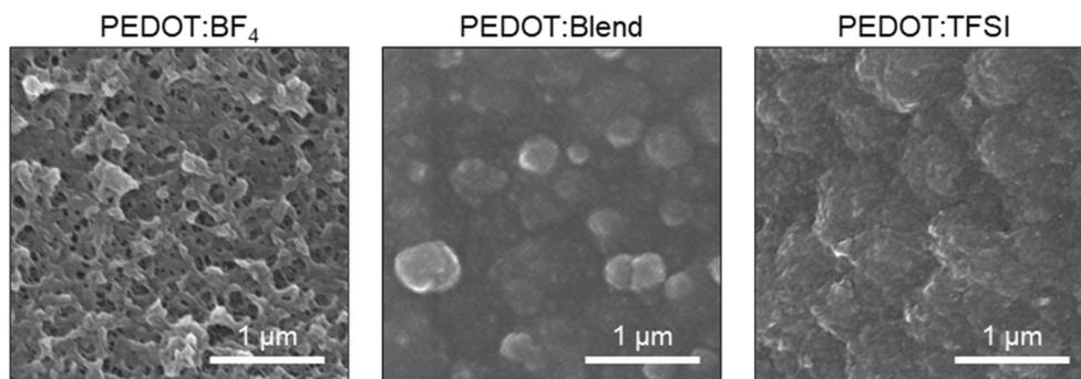
**Fig. S3** High-resolution SEM images of OSIEPed films for PEDOT:BF<sub>4</sub>, PEDOT:Blend, and PEDOT:TFSI.
