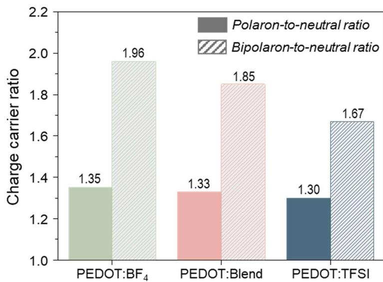
**Fig. S8** Charge carrier ratios ( $P/N$  and  $B/N$ ) of the three OSIEPed films.
