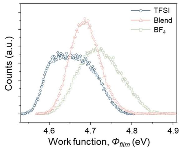
**Fig. S5** Histogram of the surface potential variations obtained by KPFM analysis.
