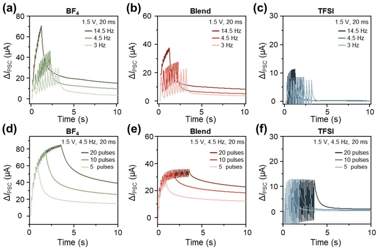
**Fig. S9** Spike rate-dependent characteristics of the (a) PEDOT:BF<sub>4</sub>, (b) PEDOT:Blend, and (c) PEDOT:TFSI synaptic transistors. Spike number characteristics of the (a) PEDOT:BF<sub>4</sub>, (b) PEDOT:Blend, and (c) PEDOT:TFSI synaptic transistors.
