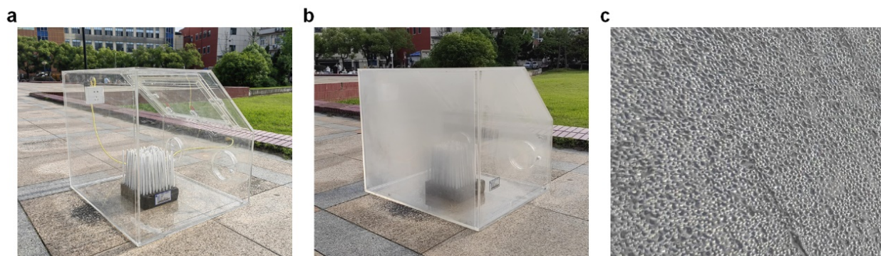
Figure S15. (a) A desalter array with a condensing shell, and (b, c) the condensed water on its surface, confirming its enormous potential in freshwater production.
