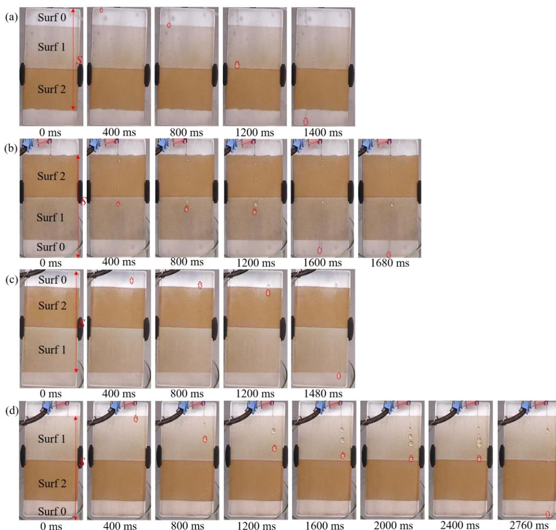
**Fig. S5** Macroscopic views of water flow on wettability-patterned surfaces. Ordered wettability-patterned surfaces (a-b). Disordered wettability-patterned surfaces (c-d).
