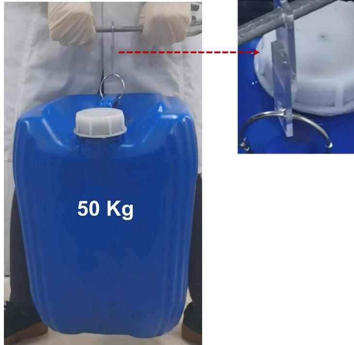
Figure S17. Lap joint area with adhesive curing underwater for 5 minutes can bear 50 Kg weight.
