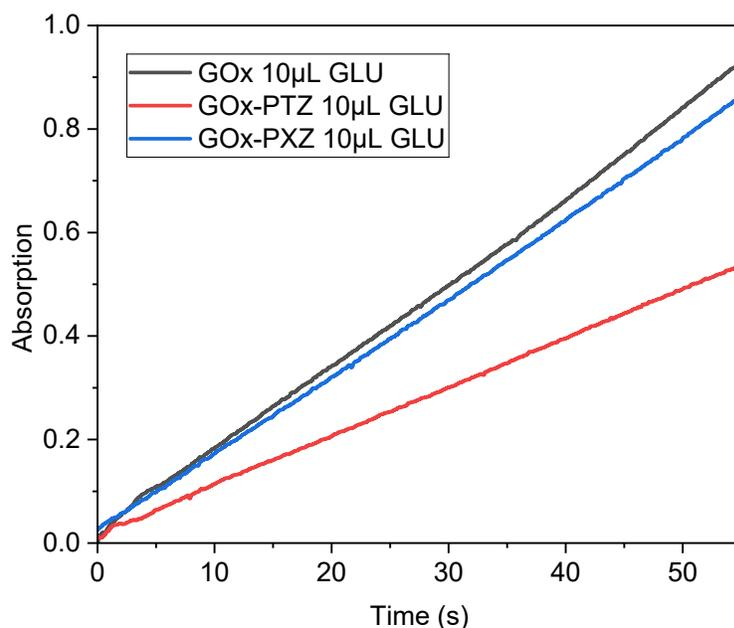
Figure S2. Biocatalytic activity curves of 10  $\mu\text{L}$  of the native GOx, and the GOx-PTZ, GOx-PXZ bioconjugates ( $1.0 \text{ mg mL}^{-1}$ ) in a cuvette consisted of 10  $\mu\text{L}$  of a solution 20 mM *o*-dianizidine, 50  $\mu\text{L}$  of  $5 \text{ mg mL}^{-1}$  HRP, 10  $\mu\text{L}$  of GLU solution (1.0 M), and PPB (50 mM, pH 7.0) added to 2 mL total volume
