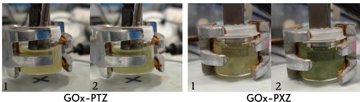
Figure S1. Illustrations of the electrochemical reaction mixtures with the electrodes before reaction (1) and after reaction (2) for the synthesis of GOx-PTZ(SO) and GOx-PXZ, respectively
