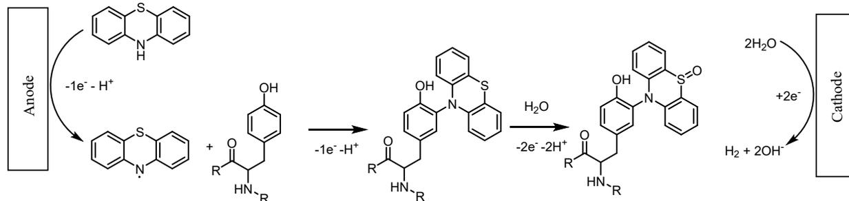
Scheme S1. Mechanism of the electrochemical reaction of the GOx-PTZ(SO) bioconjugate on anode and cathode
