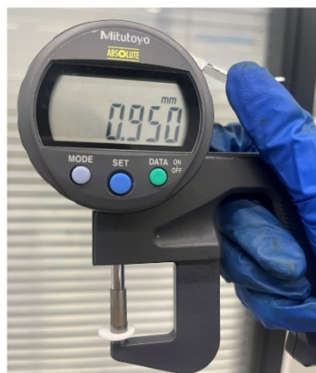
Fig. S1 The thickness of (a) pristine LAGP and (b) the polymer-coated LAGP.
