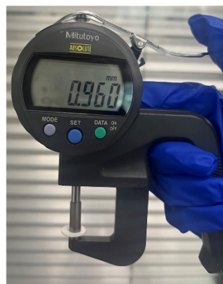
Fig. S1 The thickness of (a) pristine LAGP and (b) the polymer-coated LAGP.
