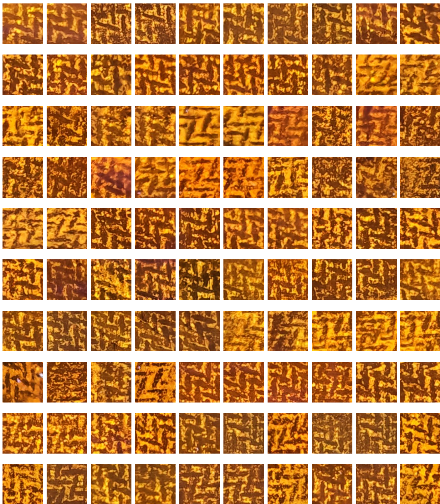
Figure S26. The image set of the surface textures of rubber inputted into CNN model for training and recognition, containing 100 fluorescent patterns recorded by MNIMP films. Photographs were taken by a built-in camera of a smartphone in a dark box with 365 nm UV irradiation.
