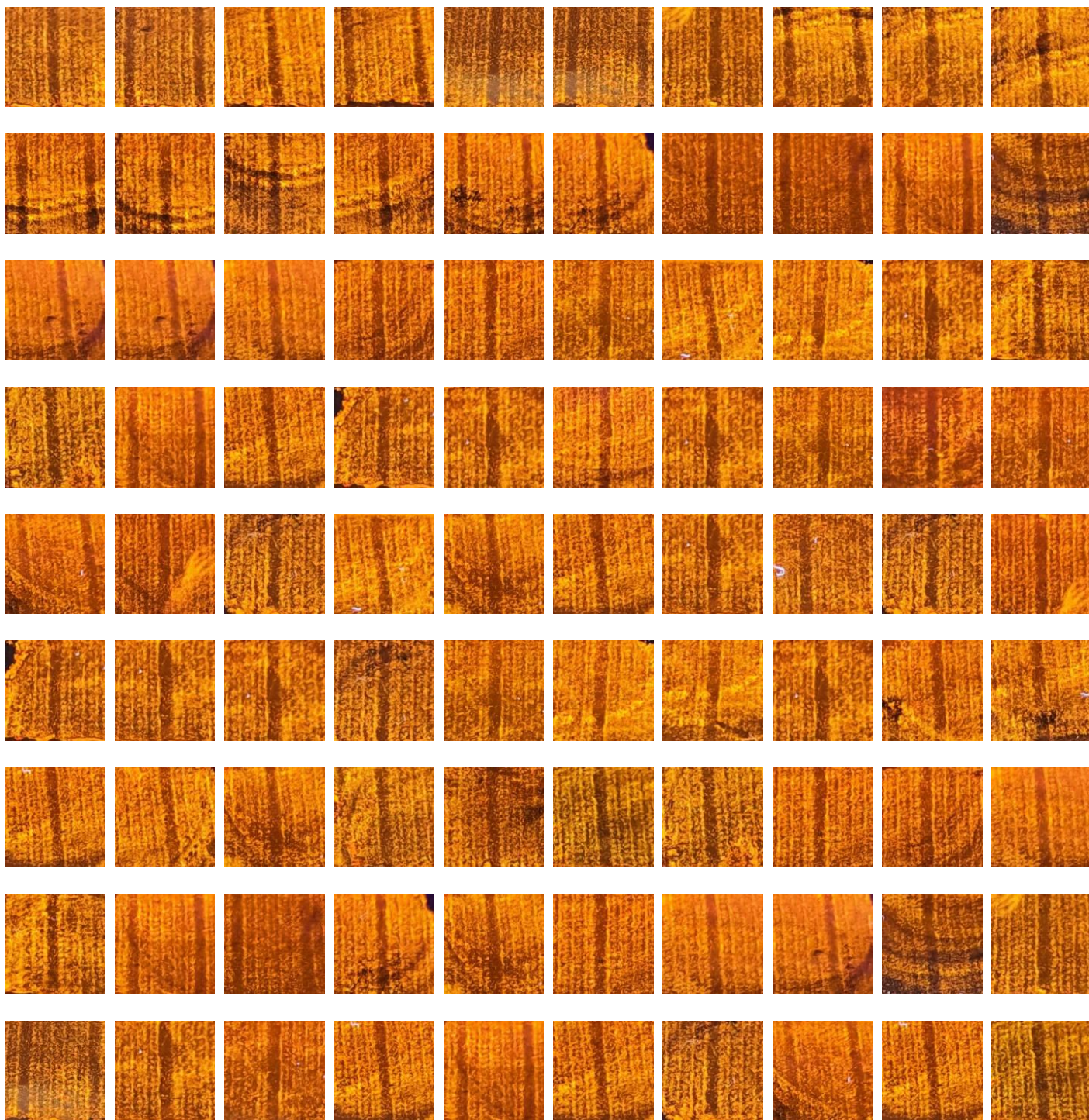
Figure S16. The image set of the surface textures of polyester inputted into CNN model for training and recognition, containing 90 fluorescent patterns recorded by MNIMP films. Photographs were taken by a built-in camera of a smartphone in a dark box with 365 nm UV irradiation.
