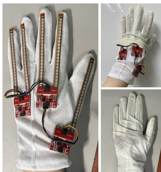
Figure S19. Demonstration of a data glove with integrated flexible strain sensors.
