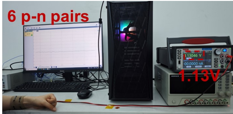
Fig. S37 Photo for the i-TE fabric with 6 p-n pairs worn on the arm.
