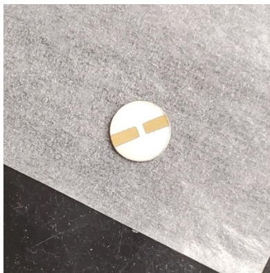
Figure S13. The pellets used for laser-driven EIS experiments. The sputtered gold electrodes demonstrate the in-plane electrode geometry where the light excitation was focused directly between the two electrodes.
