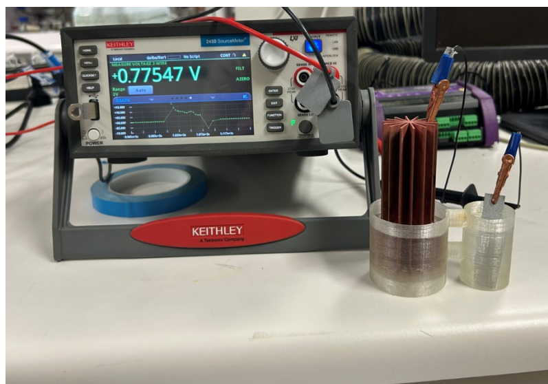
Figure S23. Setup for open-circuit voltage output and short-circuit current test using Keithley
