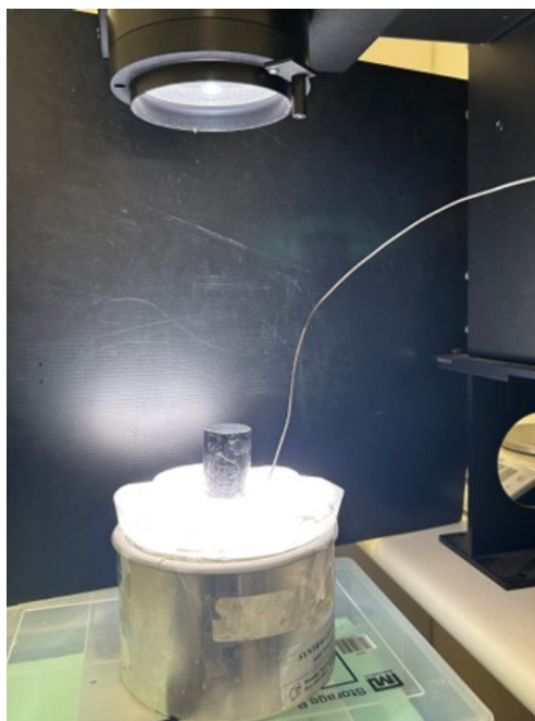
Figure S16. Photograph of the thermal-insulation system during the solar evaporation test for bulk water temperature change measurement.
