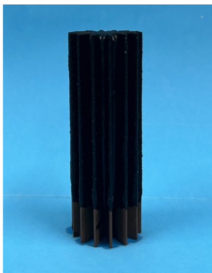
Figure S26. Photograph of Cu-evaporator-14F-15m after 8 hours solar evaporation test in real seawater. There is no salt accumulation on the surface.
