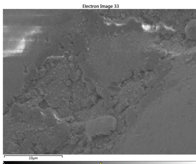
*Figure 12. SEM/EDX image of 5% w/w Na/NaCl prepared in a Schlenk flask, 10 μm scale bar.*
