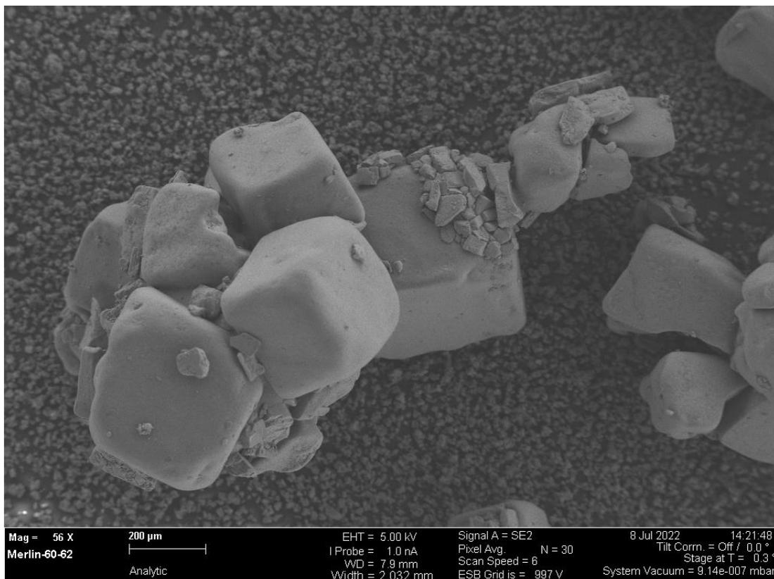
*Figure S6. SEM image of 5% w/w Na/NaCl prepared in a Schlenk flask. 56 x magnification, 200 μm scale bar.*
