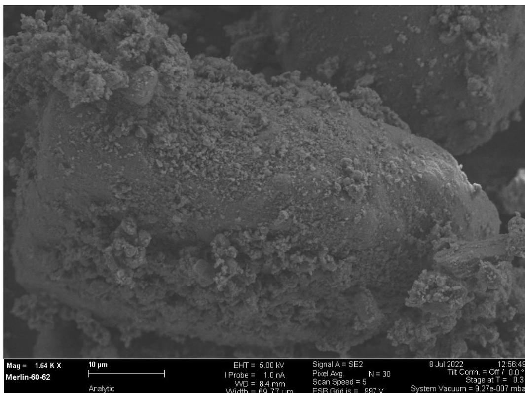
**Figure S3.** SEM image of 5% w/w Na/NaCl prepared in a planetary ballmill (Retsch PM100). 1.64 K x magnification, 10 µm scale bar.
