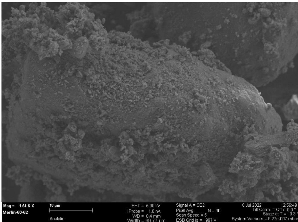
*Figure S2. SEM image of 5% w/w Na/NaCl prepared in a planetary ballmill (Retsch PM100). 1.64 K x magnification, 10 µm scale bar.*
