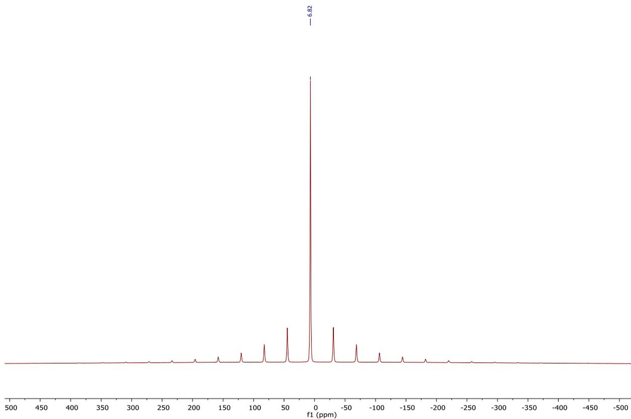
**Figure S21.**  $^{23}\text{Na}$  SS-NMR spectrum (264.63 MHz, 294.6 K, 10 KHz MAS) for 5% w/w Na/NaCl, displaying the expanded NaCl region.
