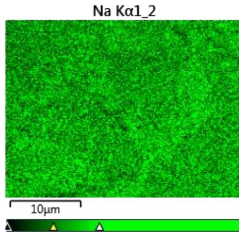
Figure S13. EDX mapping of Na on the sample illustrated in Figure 12.
