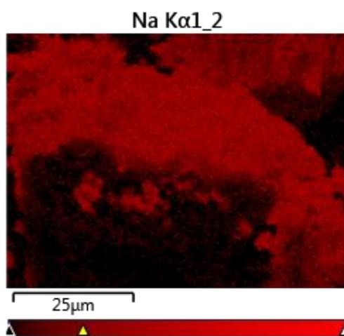
*Figure S9. EDX mapping of Na on the sample illustrated in Figure 8.*
