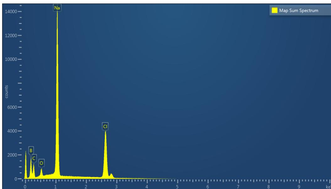
*Figure S11.EDX spectrum corresponding to **Figure 8**, showing elemental composition of material.*
