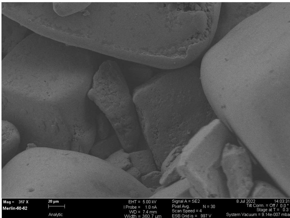
*Figure S7. SEM image of 5% w/w Na/NaCl prepared in a Schlenk flask. 317 x magnification, 20  $\mu$ m scale bar.*
