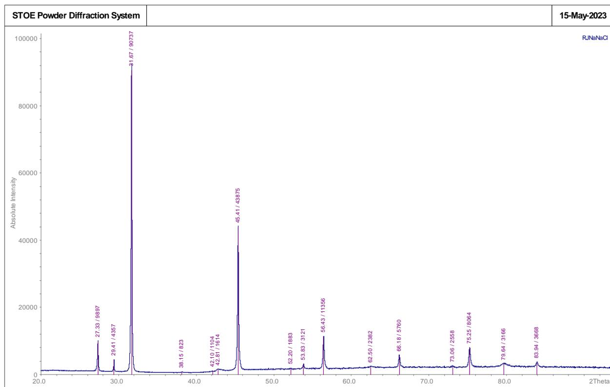
Figure S26. Powder X-ray Diffraction Pattern for 5% w/w Na/NaCl.
