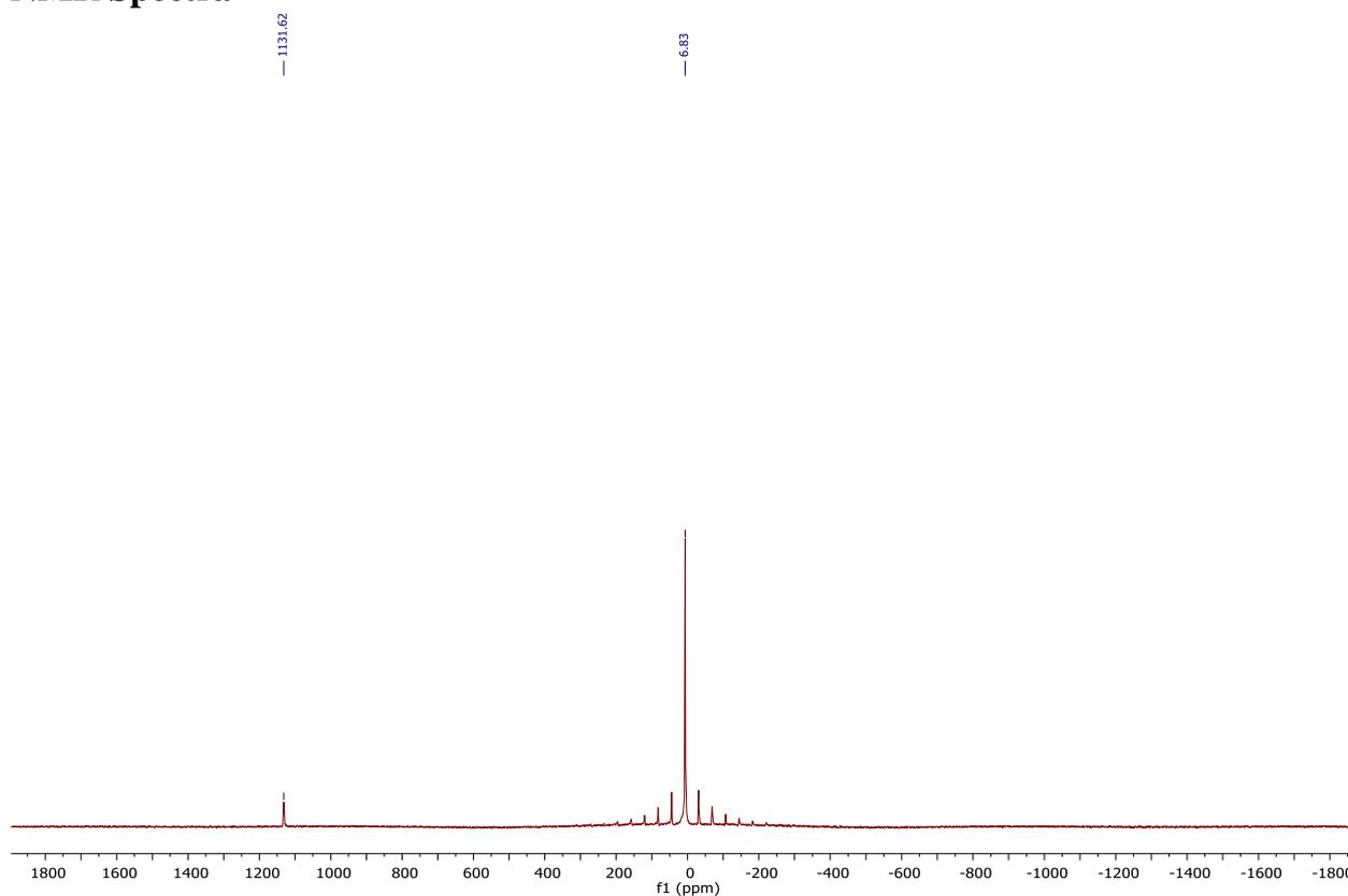
*Figure S20. <sup>23</sup>Na SS-NMR spectrum (264.63 MHz, 294.6 K, 10 KHz MAS) for 5% w/w Na/NaCl.*
