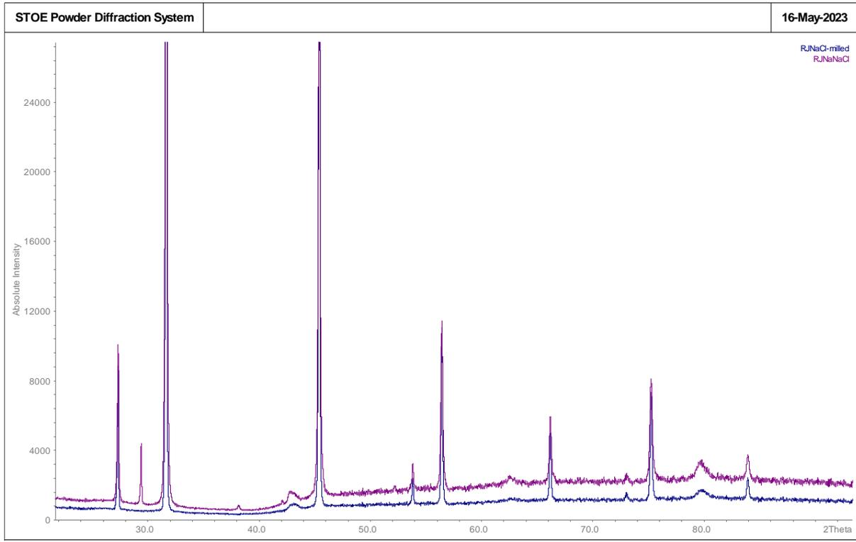
**Figure S27.** Powder X-ray Diffraction Pattern for 5% w/w Na/NaCl overlaid on top of the pattern for NaCl.
