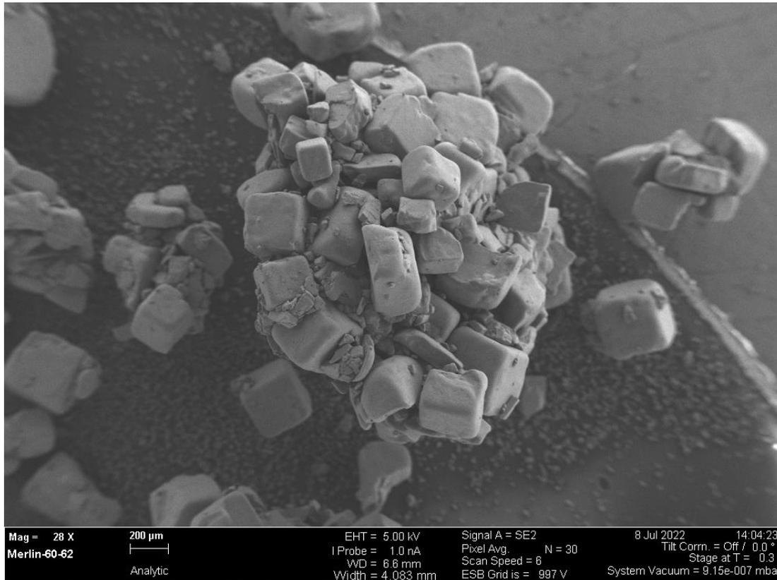
*Figure S5. SEM image of 5% w/w Na/NaCl prepared in a Schlenk flask. 28 x magnification, 200 μm scale bar.*
