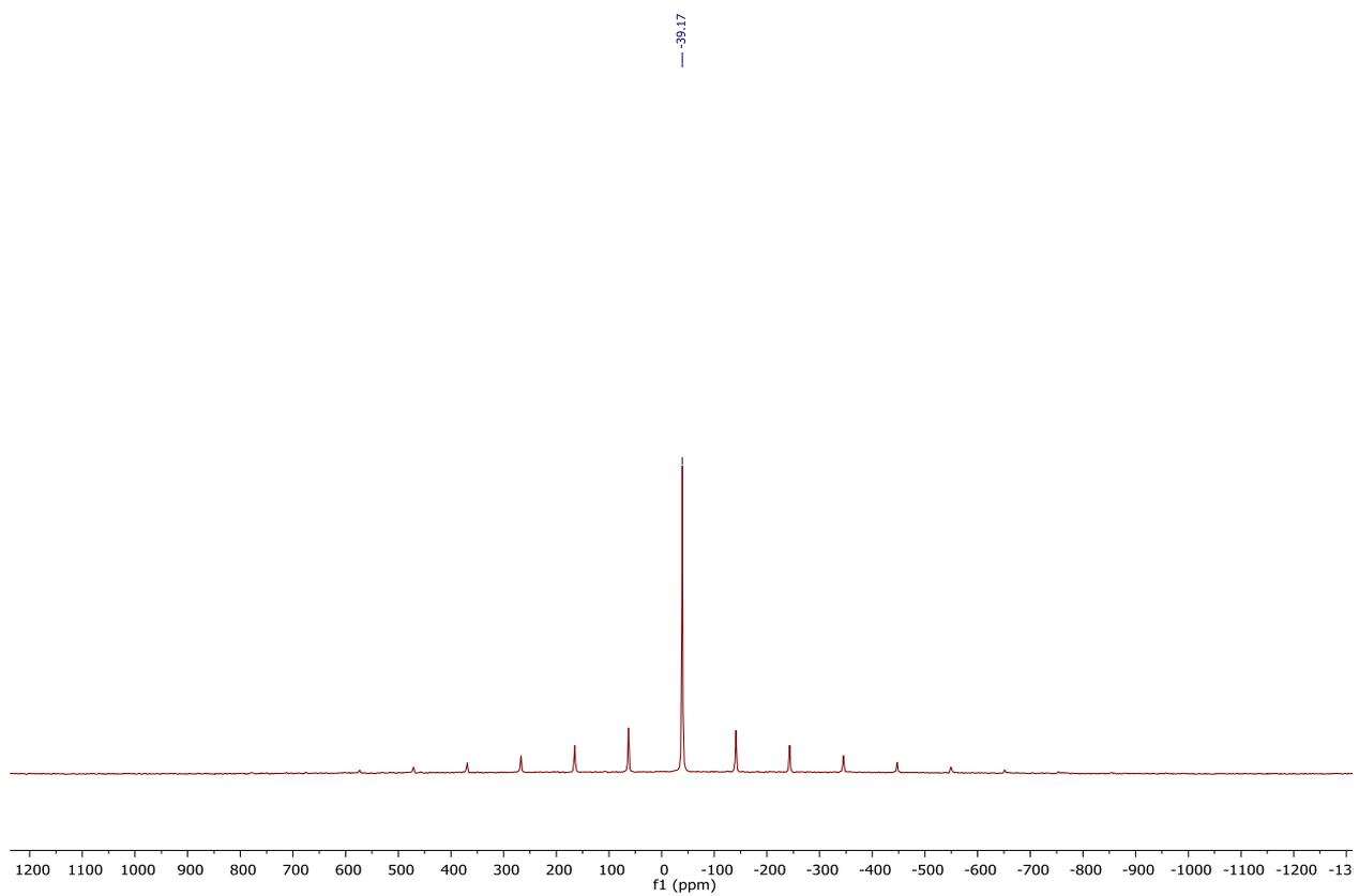
**Figure S22.**  $^{35}\text{Cl}$  SS-NMR spectrum (98.01 MHz, 294.6 K, 10 KHz MAS) for 5% w/w Na/NaCl.
