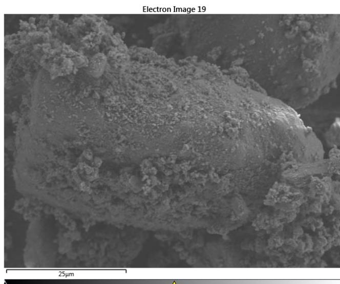
*Figure S8. SEM/EDX image of 5% w/w Na/NaCl prepared in a Ball Mill, 25 μm scale bar.*
