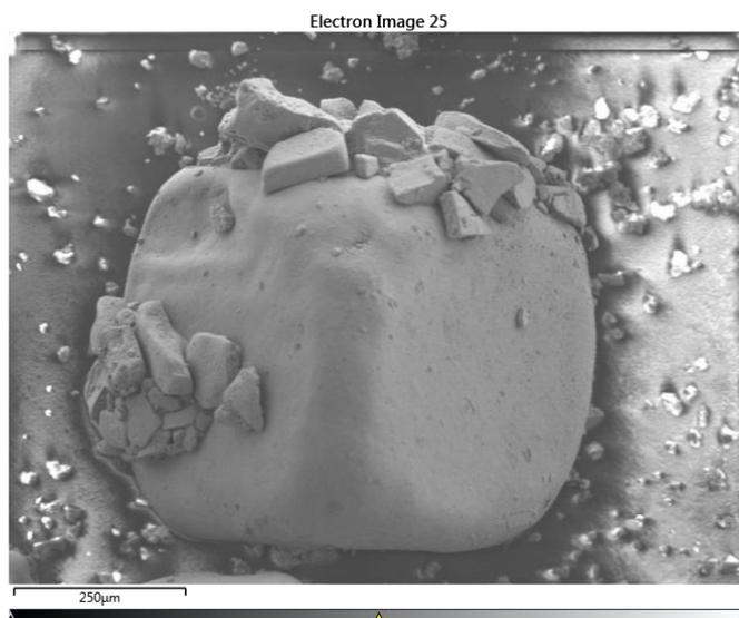
*Figure S16. SEM/EDX image of 5% w/w Na/NaCl prepared in a Schlenk flask, 250 μm scale bar.*
