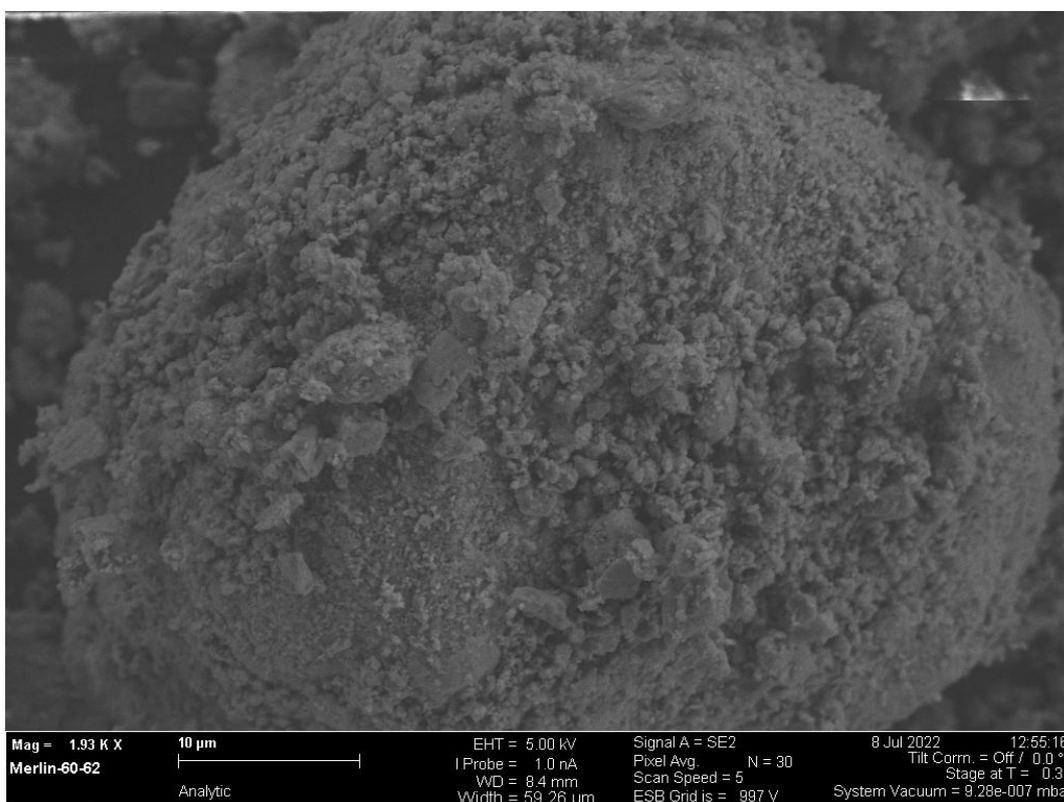
**Figure S4.** SEM image of 5% w/w Na/NaCl prepared in a planetary ballmill (Retsch PM100). 1.93 K x magnification, 10 µm scale bar.
