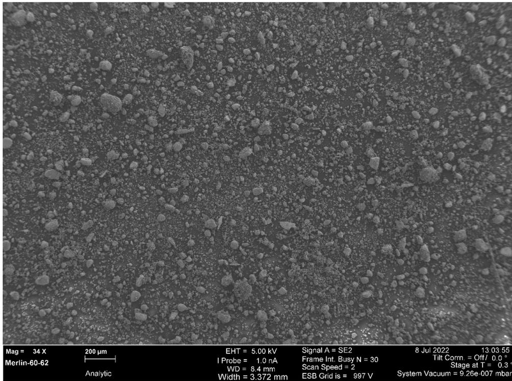
*Figure S1. SEM image of 5% w/w Na/NaCl prepared in a planetary ballmill (Retsch PM100). 34 x magnification, 200 µm scale bar*
