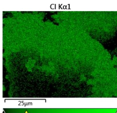
*Figure 10. EDX mapping of Cl on the sample illustrated in Figure 8.*
