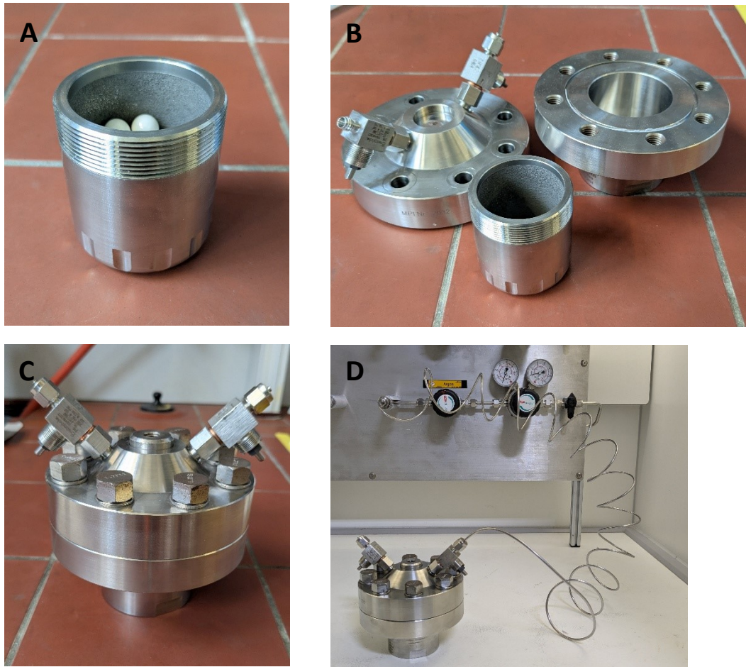
Figure S2: (a) The inlet area of custom built pressurisable stainless-steel milling (b) Top view of disassembled setup including the inner jar and the outer jacket. (c) Fully assembled and sealed stainless-steel pressure jar. (d) Experimental setup displaying the pressurized milling jar connected to the external pressure line and gauge system, used to purge the gas pressure into the jar.
