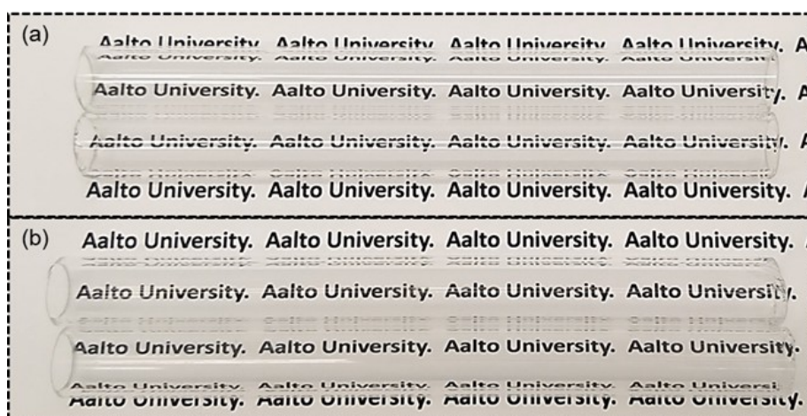
Figure S 6: Optical transparency of glass tubes. (a) Uncoated glass tube and (b) SHB nanograss-coated glass tube placed over printed text (“Aalto University”). Both tubes show transparency with the SHB coated tubes showing less reflection from ceiling lights, indicating that the SHB coating retains the antireflection property of GLA on glass and improves transparency and does not impair it.
