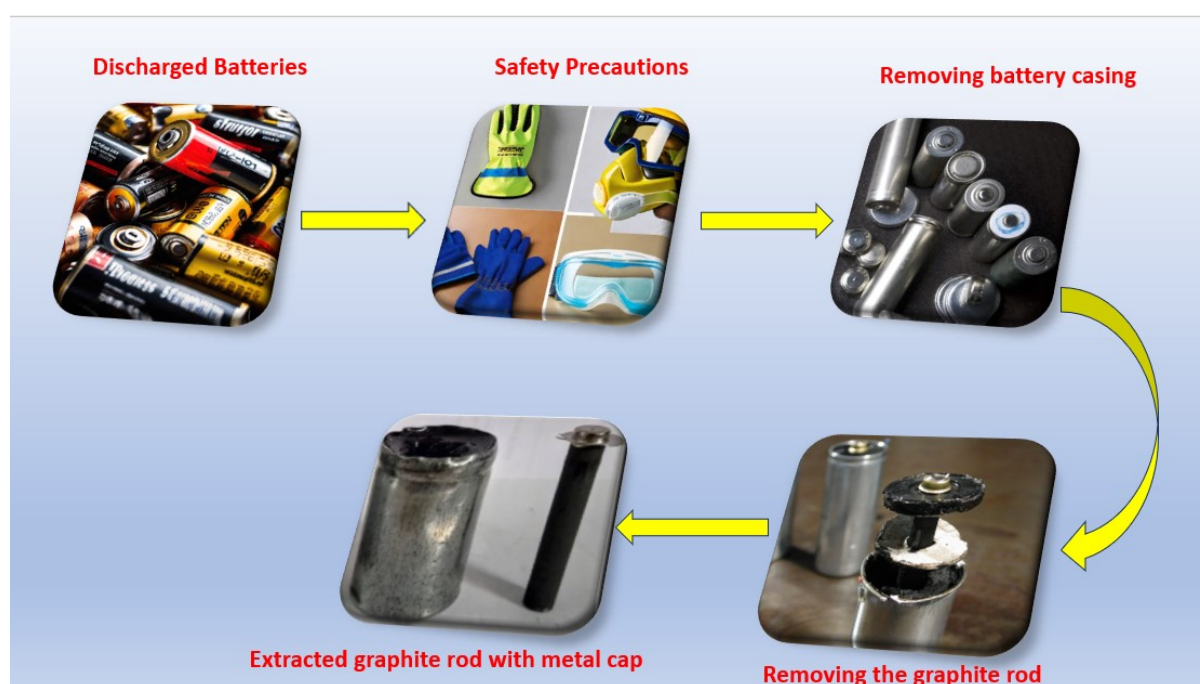
S.1 . Illustration of the safe dismantling of a graphite rod from batteries.
