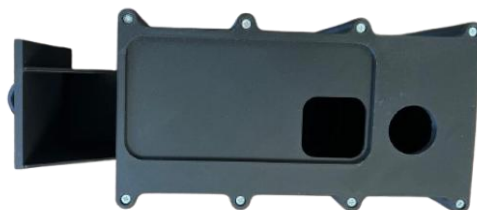
Figure S7. 3D-printed dark chamber with a drawer to insert the solid sensor, a slot for the smartphone and a hole for the UV LED.
