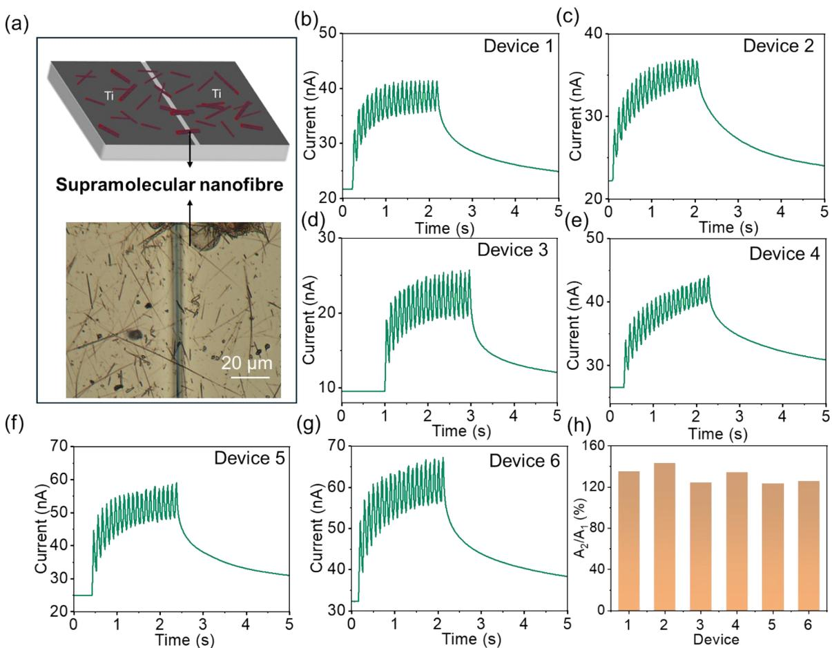
**Figure S5** (a) Schematic of the device and the optical microscopy image of the nanofibres spread across the gap between Ti electrodes. (b-g) Six devices and their photoresponse studied at 70% RH. 20 optical pulses of 50 ms pulse width ( $t_w$ ) and 50 ms pulse interval ( $t_i$ ) are applied. (h) Paired pulse facilitation (PPF) index of all the six devices.
