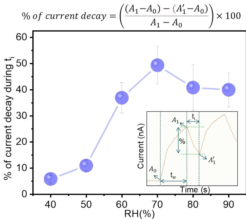
**Figure S4** % of current decay during  $t_i$  (200 ms) between optical exposure at varied RHs. Inset shows the photoresponse for two optical pulses depicting the method of % decay calculation and the equation used is shown on the top.
