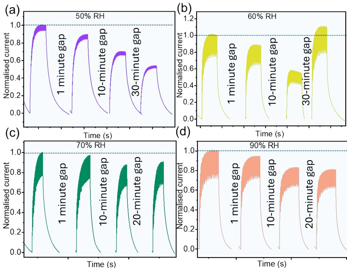
**Figure S11** Photocurrent at (a) 50% (normalized with respect to  $\sim 10.9$  nA), (b) 60% (normalized with respect to  $\sim 35.6$  nA), (c) 70% (normalized with respect to  $\sim 91.2$  nA) and (d) 90% RH (normalized with respect to  $\sim 188.2$  nA) studied by varying the time gap.
