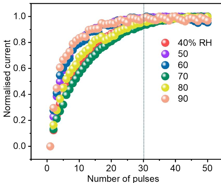
**Figure S3** Normalized current response at different RH for 50 optical pulses exhibiting saturation around 30 pulses.
