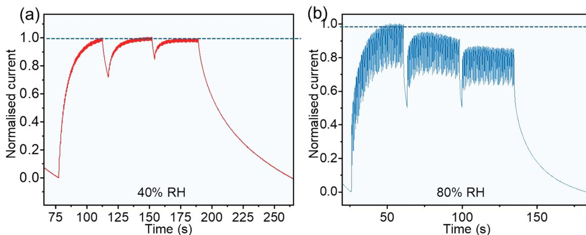
**Figure S17** Photoreponse at (a) 40% (normalized with respect to  $\sim 2$  nA) and (b) 80% RH (normalized with respect to  $\sim 90.4$  nA) with the application of 50 optical pulses consecutively.
