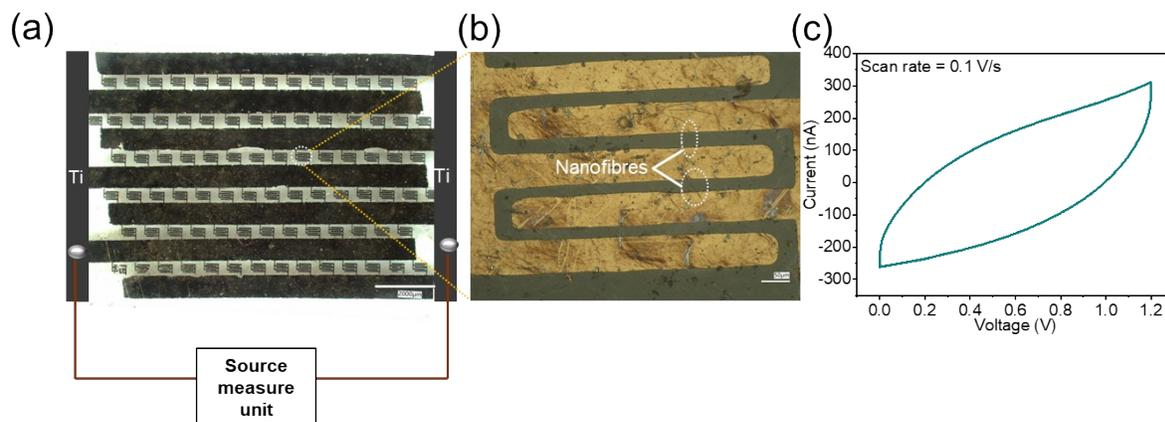
**Figure S2** (a) Optical image of the entire device connected to a source measure unit. (b) Magnified optical image showing the nanofibres spread across the interdigitated electrodes. (c) I-V sweep from 0 to 1.2 V.
