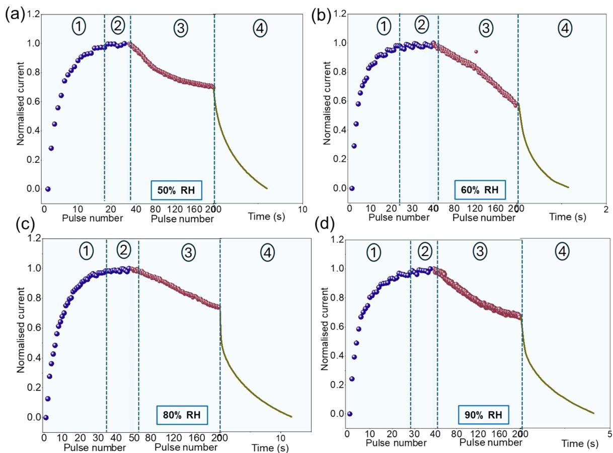
**Figure S15** Learning profile exhibited at (a) 50% (normalized with respect to  $\sim 10.8$  nA), (b) 60% (normalized with respect to  $\sim 16.6$  nA), (c) 80% (normalized with respect to  $\sim 125.1$  nA) and (b) 90% RH (normalized with respect to  $\sim 127.1$  nA). The four stages of learning are 1-potential, 2-habituation, 3-depression, and 4-spontaneous forgetting.
