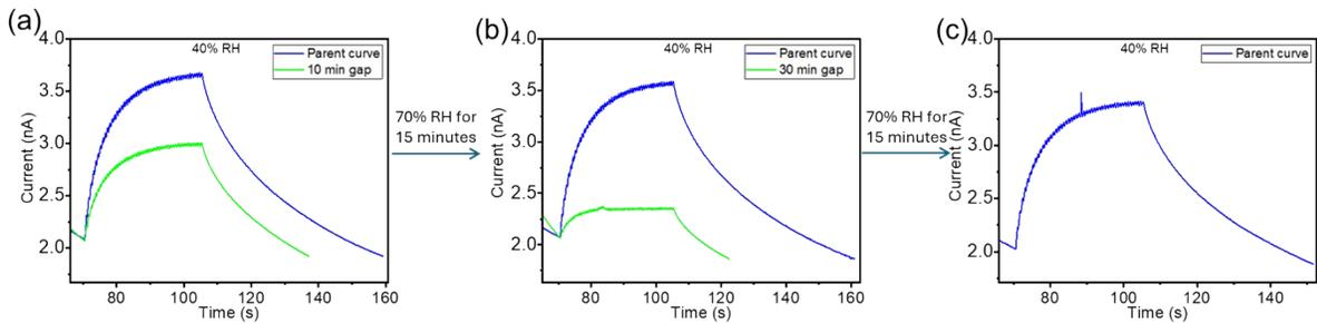
**Figure S10** (a) Optical response at 40% RH for 50 pulses with the parent curve (blue) and the curve after 10 minutes time gap (green). (b) Recovery of the optical response (blue curve) after exposure to 70% RH for 15 minutes and the decrease in photoresponse with 30 minutes time gap (green curve). (c) Recovery of the photoresponse again after exposure to 70% RH for 15 minutes.
