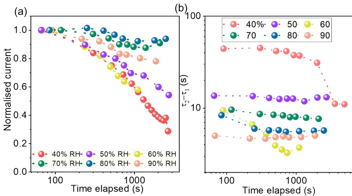
**Figure S12** Variation in (a) current and (b) consolidation parameter  $\tau_2 - \tau_1$  with time at different RH.
