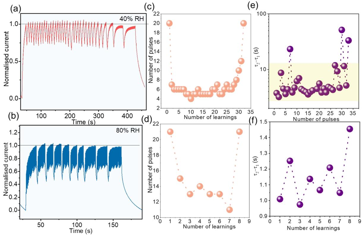
**Figure S9** Learning-forgetting-relearning emulated at (a) 40% (normalized with respect to  $\sim 1.6$  nA) and (b) 80% RH (normalized with respect to  $\sim 58.8$  nA) with the initial learning performed with 20 pulses. Number of pulses required for consecutive learnings at (c) 40% and (d) 80% RH. The variation of  $\tau_2 - \tau_1$  (consolidation parameter) with the learning process at (e) 40% and (f) 80% RH.
