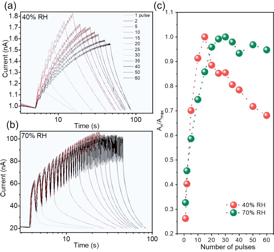
**Figure S13** Photoresponse with increasing number of pulses at (a) 40% and (b) 70% RH. (c) Variation in photoresponse with the increase in the number of pulses at 40 and 70% RH.
