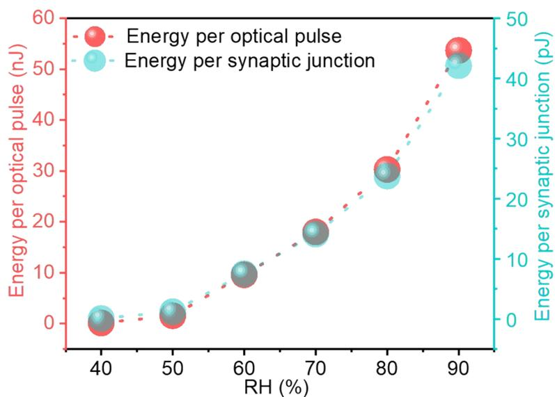
**Figure S6** Energy consumption per optical pulse (red curve) and per synaptic junction (blue curve) at different RHs.
