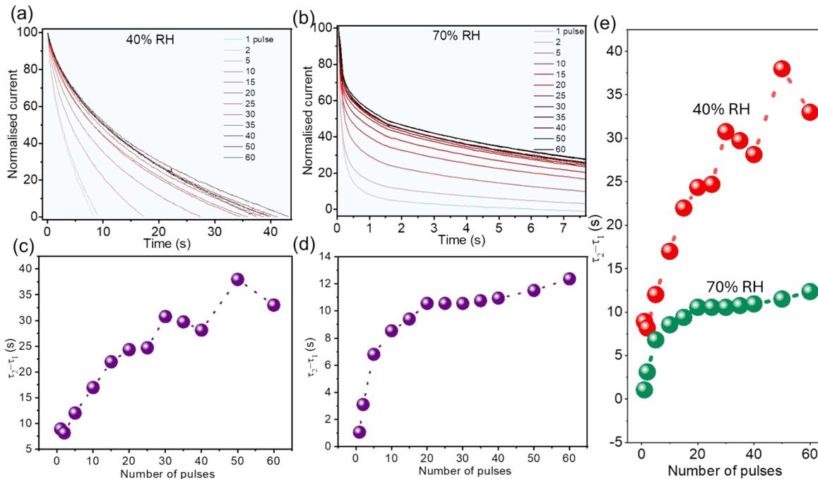
**Figure S14** Decay curves with varying number of pulses at (a) 40% and (b) 70% RH. Variation in the consolidation parameter  $\tau_2 - \tau_1$  at (c) 40% and (d) 70% RH. (e) Comparison of variation in the consolidation parameter at 40 and 70% RH.
