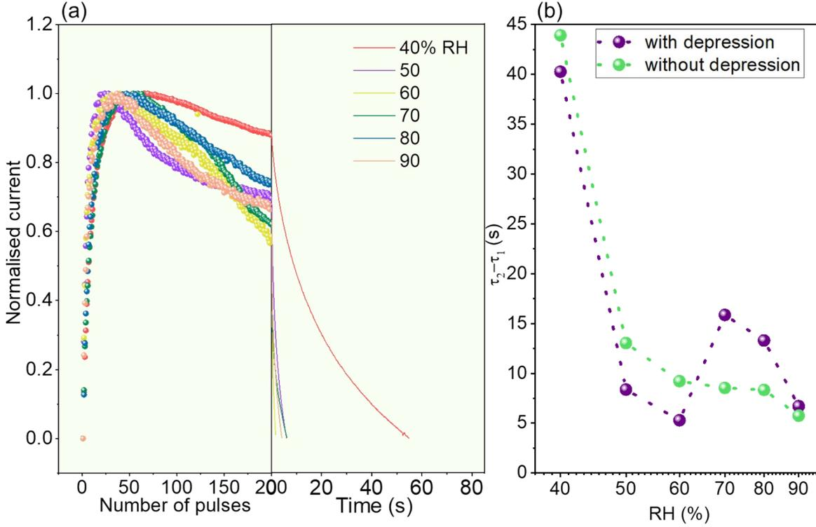
**Figure S16** (a) Photocurrent and decay variation with RH during the application of 200 pulses. (b) Comparison of the consolidation parameter variation ( $\tau_2 - \tau_1$ ) without and with depression behavior, as observed in Figures 2c and 5e, respectively.
