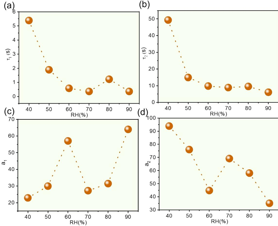
**Figure S7** The variation of the parameters (a)  $\tau_1$  (b)  $\tau_2$  (c)  $a_1$  and (d)  $a_2$  with increasing RH for the decay after the application of 50 optical pulses.
