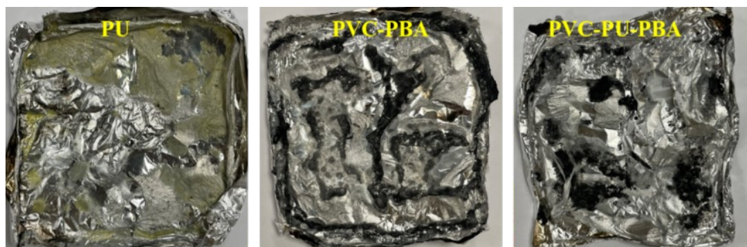
Fig. S4. Digital photographs of char residues of PU, PVC-PBA, and PVC-PU-PBA after the cone calorimeter test.
