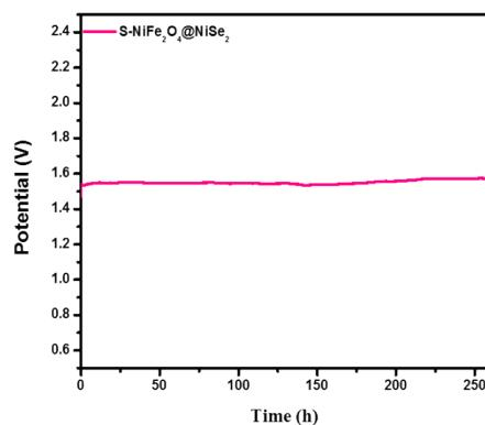
Figure S8 The V-t curve of S-NiFe<sub>2</sub>O<sub>4</sub>@NiSe<sub>2</sub> for OER at 50 mA cm<sup>-2</sup>.
