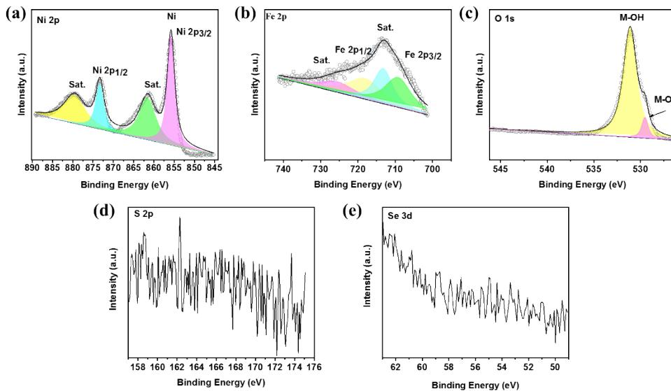
Figure S9 High resolution XPS spectra of Ni 2p (a), Fe 2p (b), O 1s (c), S 2p (d) and Se 3d in S-NiFe<sub>2</sub>O<sub>4</sub>@NiSe<sub>2</sub> electrocatalyst after OER stability test.
