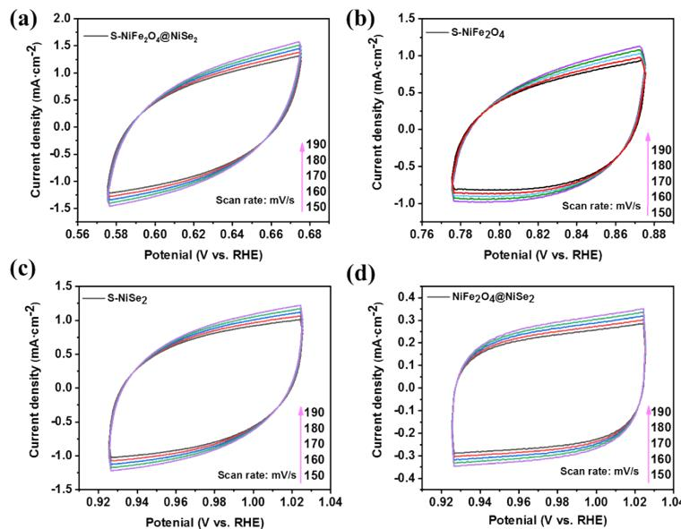
Figure S7 Cyclic voltammetry curves of S-NiFe<sub>2</sub>O<sub>4</sub>@NiSe<sub>2</sub>, S-NiFe<sub>2</sub>O<sub>4</sub>, S-NiSe<sub>2</sub>, and NiFe<sub>2</sub>O<sub>4</sub>@NiSe<sub>2</sub> electrocatalysts with the scan rate of 150-190 mV s<sup>-1</sup> in non-Faradic region.
