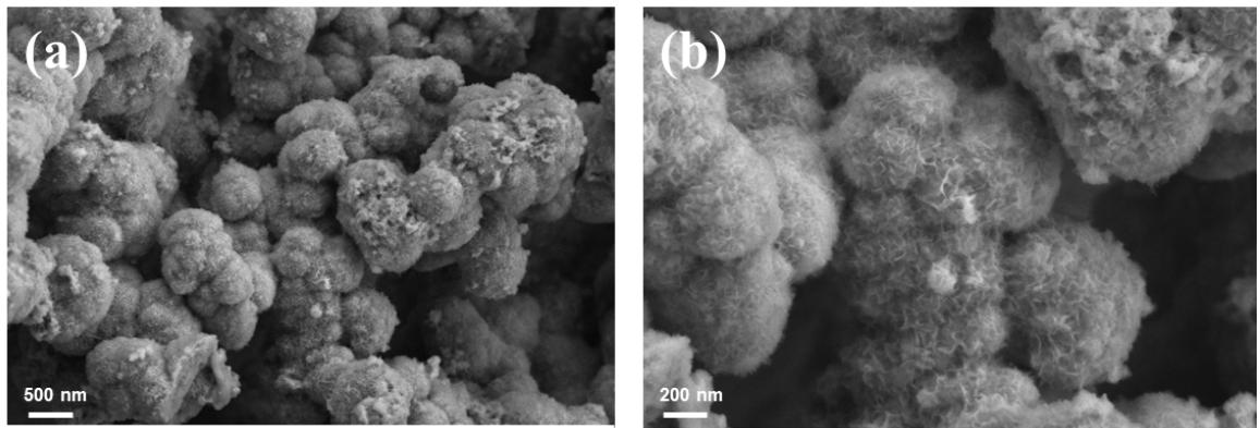
Figure S3 SEM images of S-NiFe<sub>2</sub>O<sub>4</sub>@NiSe<sub>2</sub> electrocatalyst after OER stability test.
