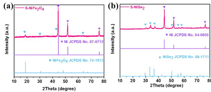
Figure S6 XRD patterns of S-NiFe<sub>2</sub>O<sub>4</sub> and S-NiSe<sub>2</sub> electrocatalysts.
