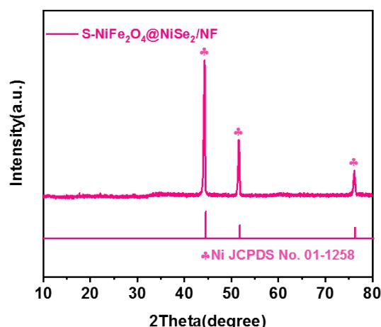
Figure S1 XRD pattern of S-NiFe<sub>2</sub>O<sub>4</sub>@NiSe<sub>2</sub>/NF electrocatalyst after OER stability test.
