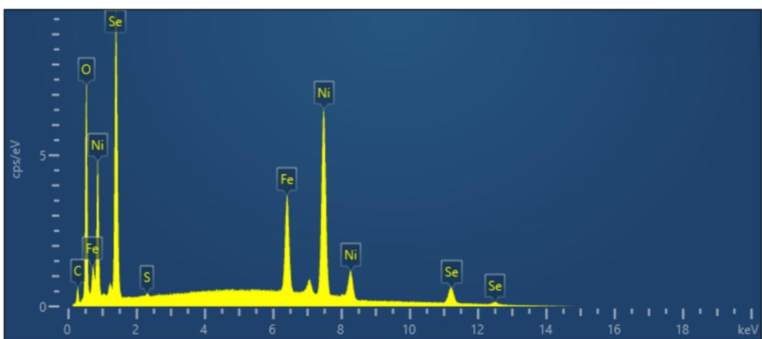
Figure S4 EDS spectrum of S-NiFe<sub>2</sub>O<sub>4</sub>@NiSe<sub>2</sub> electrocatalyst.
