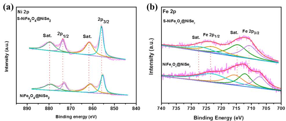
Figure S5 XPS spectra of Ni 2p (a) and Fe 2p (b) of S-NiFe<sub>2</sub>O<sub>4</sub>@NiSe<sub>2</sub> and NiFe<sub>2</sub>O<sub>4</sub>@NiSe<sub>2</sub>.
