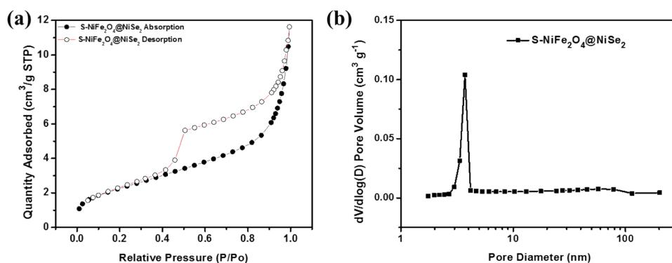
Figure S2 The N<sub>2</sub> adsorption/desorption isotherm (a) and pore-size distribution (b) of S-NiFe<sub>2</sub>O<sub>4</sub>@NiSe<sub>2</sub> electrocatalyst.
