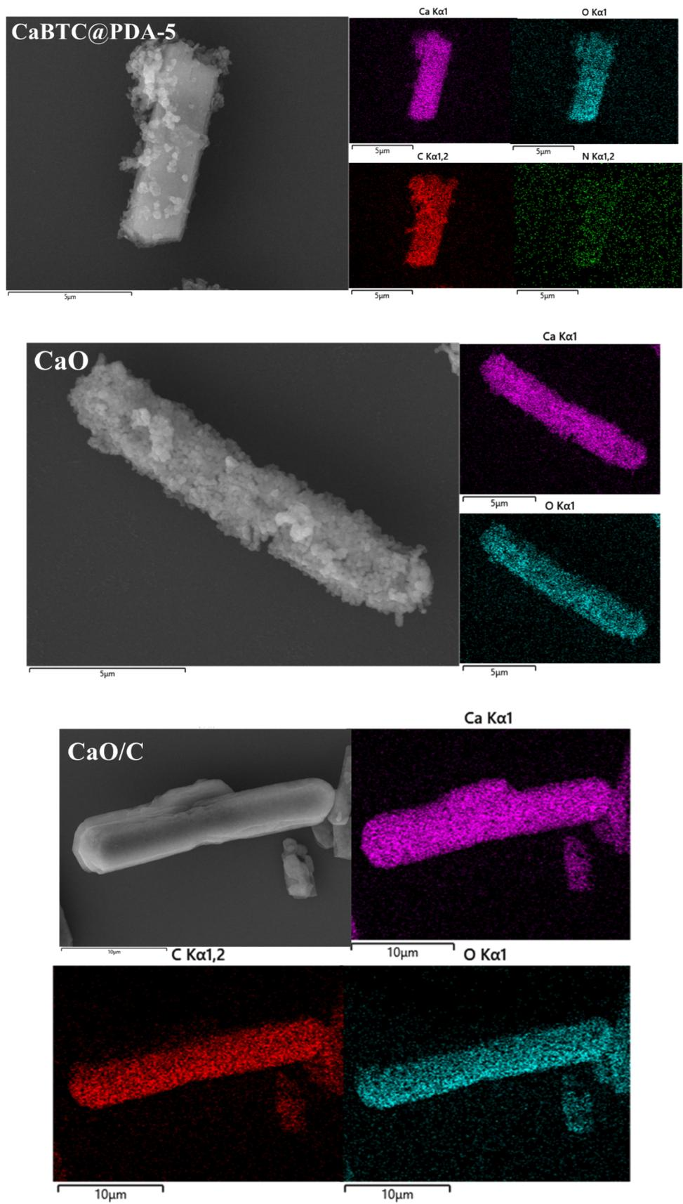
Figure S2: SEM images of Ca/CN-2 , Ca/CN-8, CaBTC@PDA-5, CaO, CaO/C and elements mapping (Ca, O, C, N) for CaBTC@PDA-5, CaO, CaO/C
