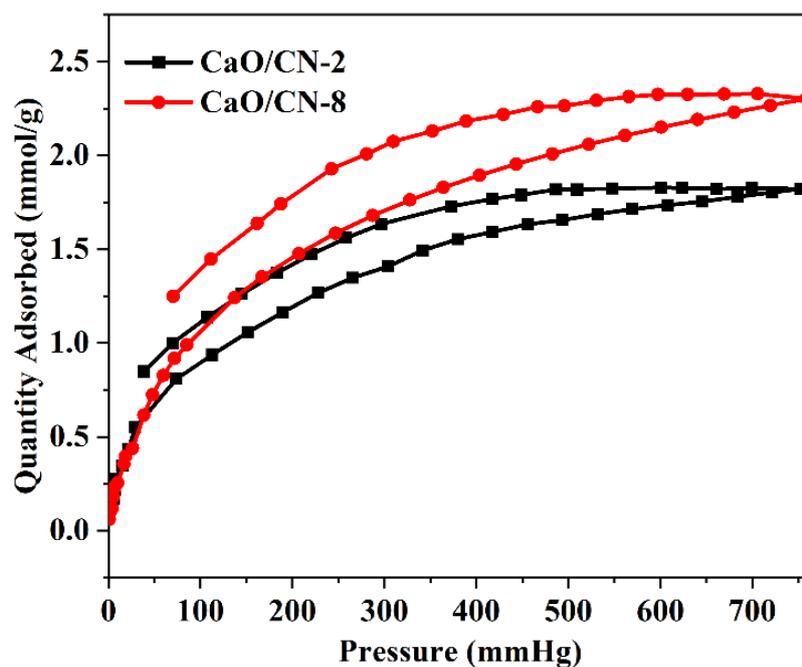
Fig. S5: CO<sub>2</sub> adsorption-desorption isotherms of Ca/CN-2 and Ca/CN-8
