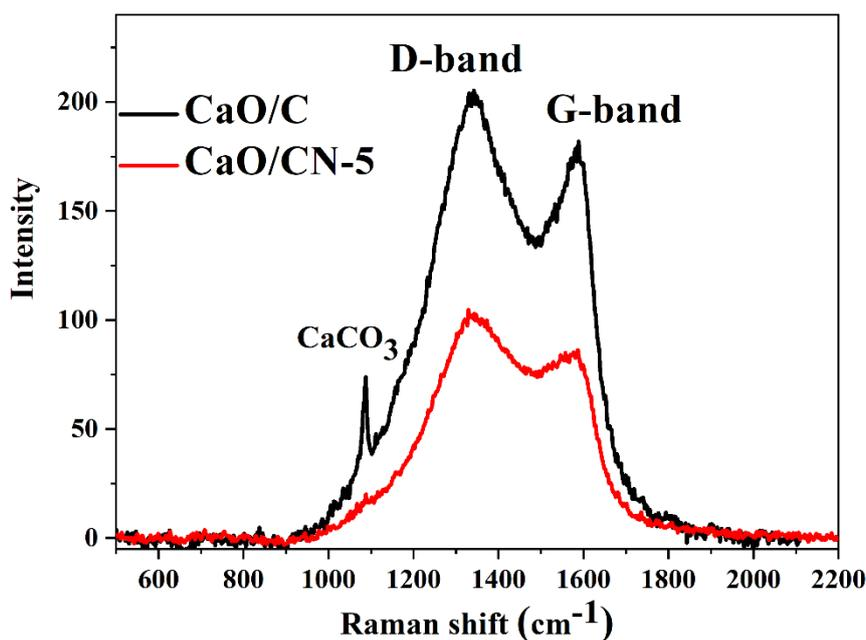
Fig. S3: Raman spectra of CaO/C and CaO/CN-5.
