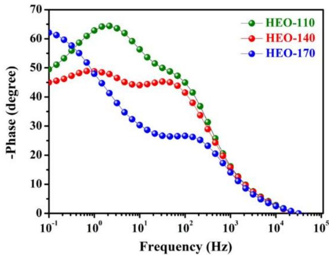
**Fig. S9** The Bode plot of the temperature varied high entropy electrode material.
