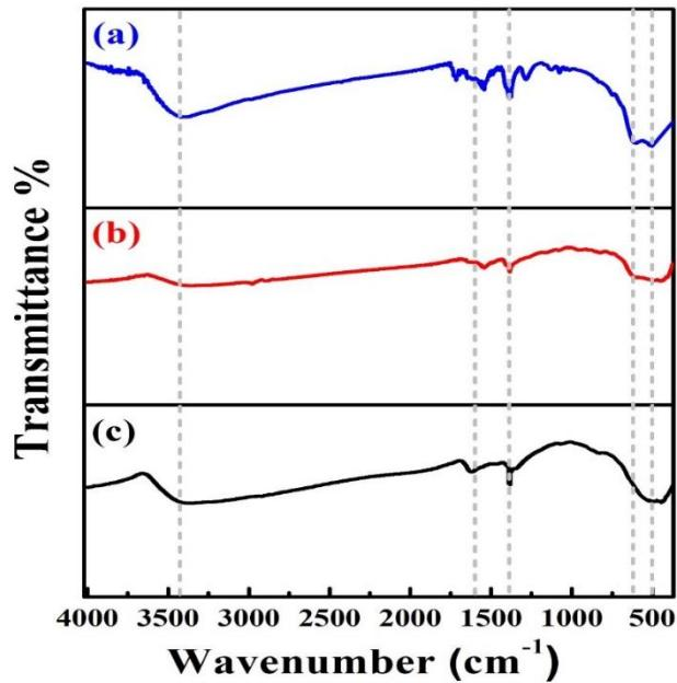
**Fig. S6** IR spectra of synthesized HEOs; HEO-170 (a), HEO-140 (b), HEO-110 (c).
