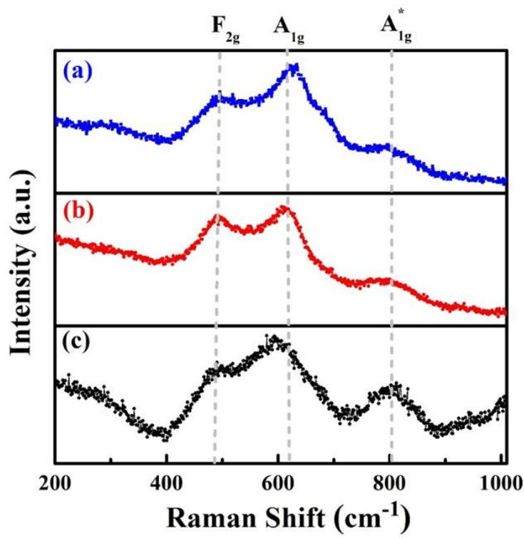
**Fig. S5** Raman spectra of synthesized HEOs; (a) HEO-170, (b) HEO-140, (c) HEO-110.
