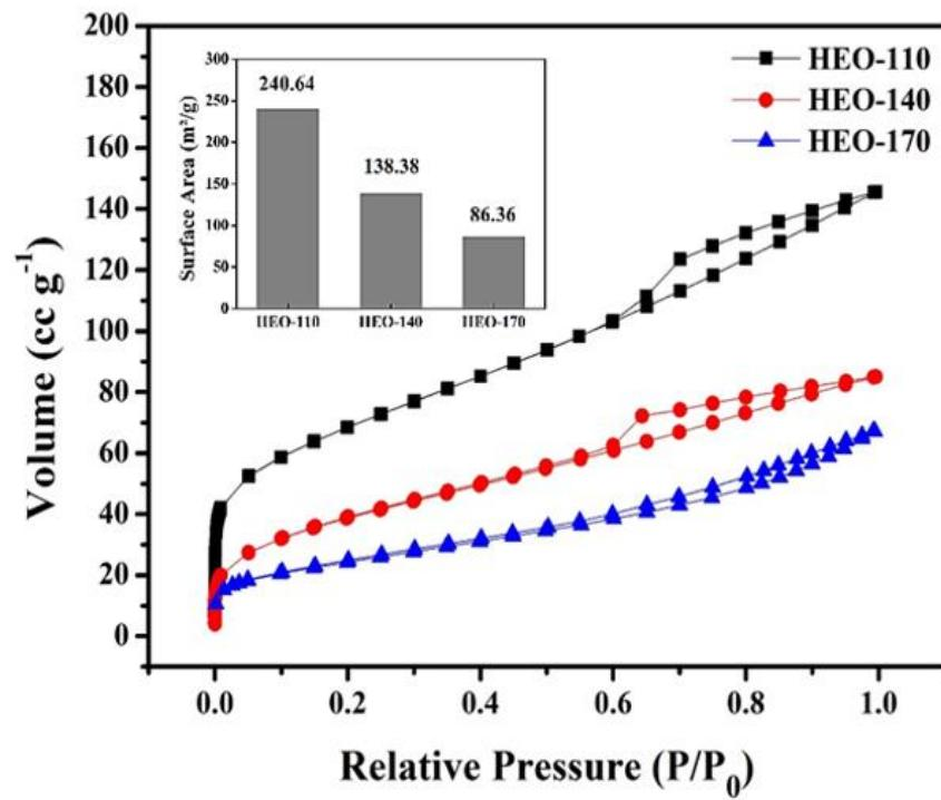
**Fig. S4** N<sub>2</sub> adsorption-desorption isotherm of HEO-110, HEO-140 and HEO-170. The inset is the BET surface area of respective HEOs.
