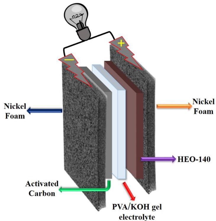
**Fig. S10** A diagrammatic representation of the fabrication of the device.
