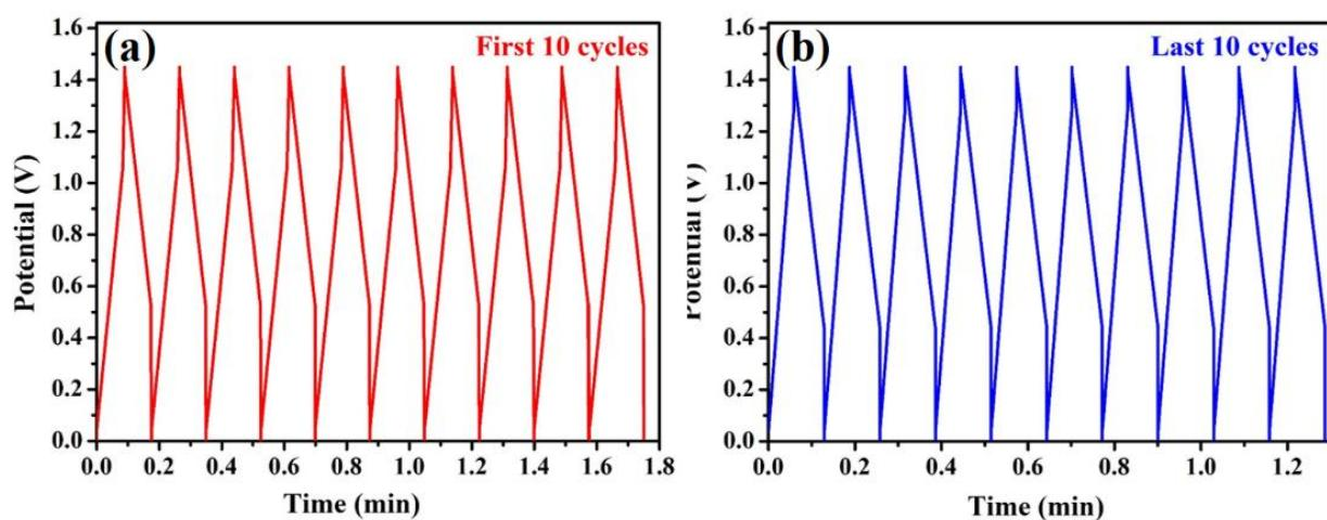
**Fig. S11** The stability data in terms of first 10 cycles and last 10 GCD cycles.
