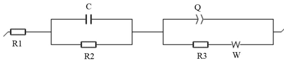
**Fig. S8** Equivalent circuit model of EIS fitting.
