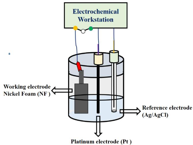
**Fig. S7** Schematic diagram for the electrochemical study of electrode materials.
