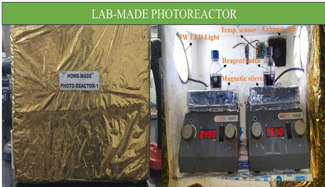
Fig. S6. Lab-made photoreactor (Outer View and Inner View)
