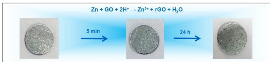
**Fig. S4** Optical photographs of Zn foil immersed in  $\text{ZnSO}_4$ -Gly-GO electrolytes.
