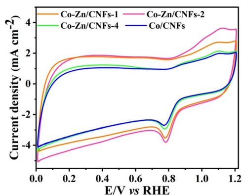
Fig. S13 CV curves of different catalysts in O<sub>2</sub>-saturated 0.1M KOH
