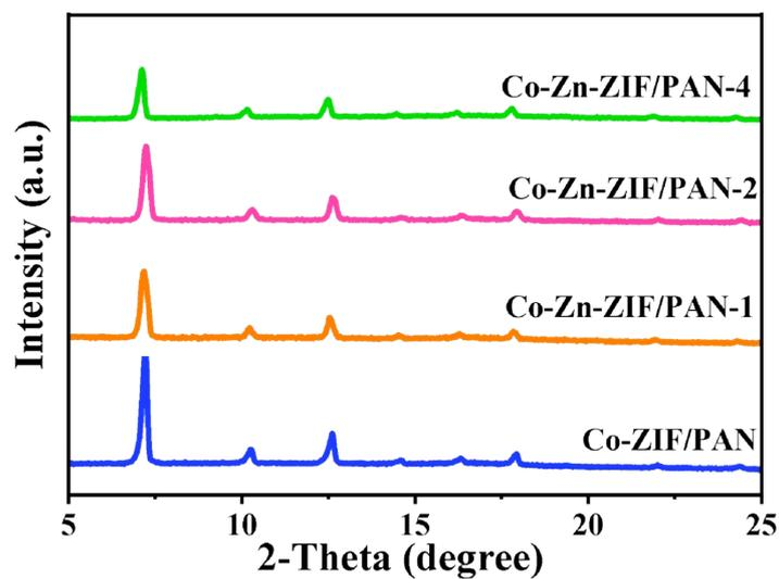
Fig. S5 XRD patterns of Co-Zn-ZIF/PAN-4, Co-Zn-ZIF/PAN-2, Co-Zn-ZIF/PAN-1 and Co-ZIF/PAN.
