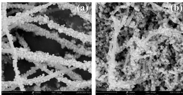
**Fig. S10** (a) and (b) SEM images of the Co-Zn/CNFs-2 before and after OER test.
