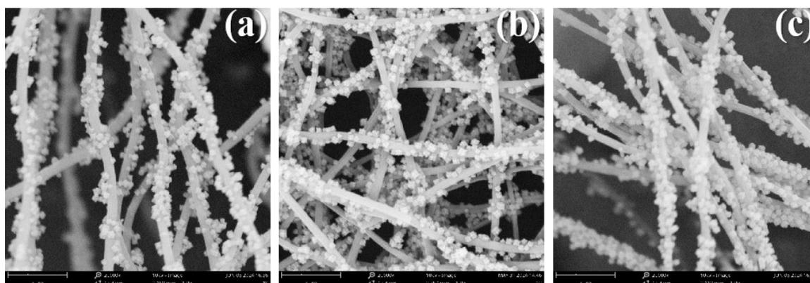
**Fig. S2** (a), (b), (c) and (d) SEM images of the Co-Zn/CNFs-4, Co-Zn/CNFs-1 and Co/CNFs, respectively.
