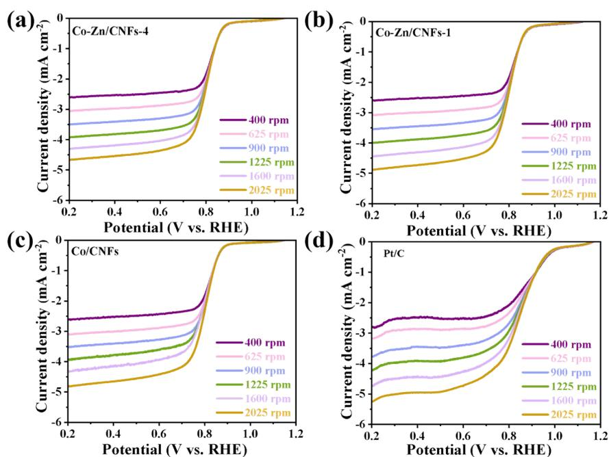
Fig. S14 (a), (b) and (c) LSV curves of Co-Zn/CNFs-4, Co-Zn/CNFs-1 and Co/CNFs samples at different rotation rates.
