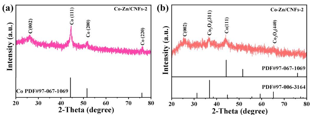
**Fig. S11** (a) and (b) XRD patterns of Co-Zn/CNFs-2 before and after OER test.
