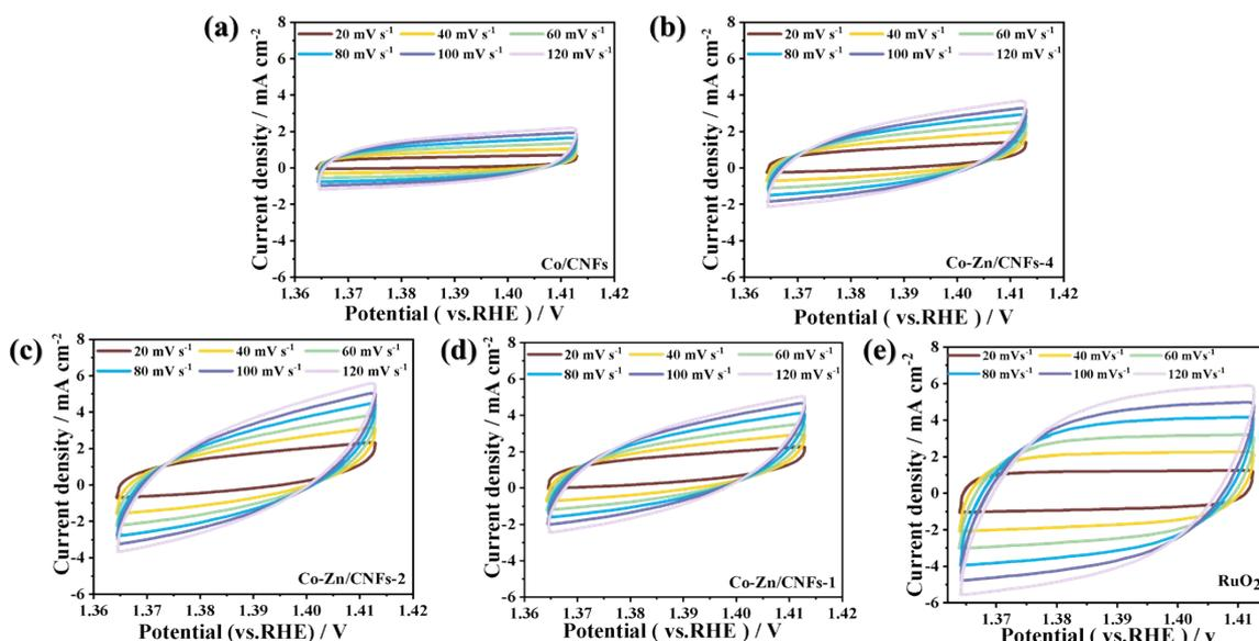
**Fig. S9** The CV measurements in a non-faradic current region of (a) Co/CNFs, (b) Co-Zn/CNFs-4, (c) Co-Zn/CNFs-2, (d) Co-Zn/CNFs-1 and (e) RuO<sub>2</sub> at different scan rates of 20, 40, 60, 80, 100, and 120 mV s<sup>-1</sup>.
