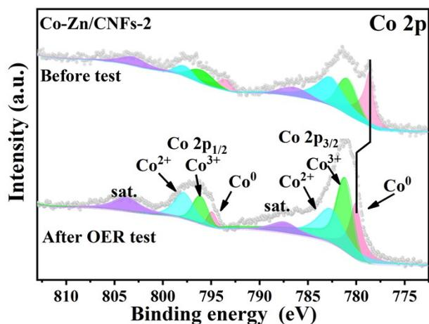
Fig. S12 XPS spectrum image of Co-Zn/CNFs-2 before and after OER test.
