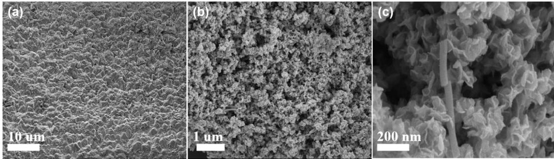
Fig.S1. SEM images of (a)  $\text{Ni}_3\text{S}_2/\text{NF}$  and (b-c)  $\text{MoS}_2$
