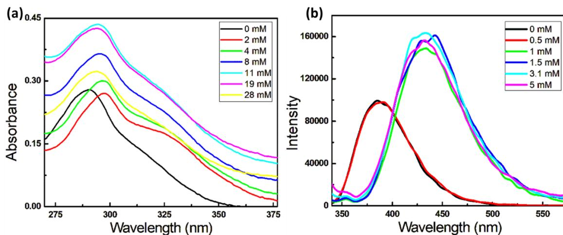
**Figure S6.** (a) absorption spectra and emission spectra ( $\lambda_{\text{exc}}$  320 nm) of EBINP in gradual addition of NaOH (0.25 M) in ACN medium.
