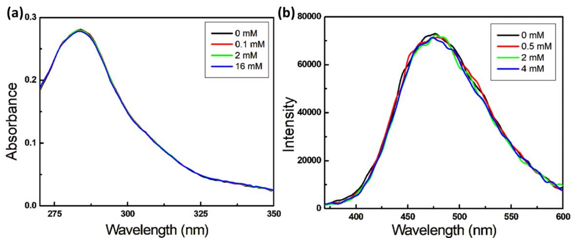
**Figure S3.** (a) absorption spectra and (b) emission spectra ( $\lambda_{\text{exc}}$  320 nm) of EBINP in gradual addition of AcOH (0.25 M) in water medium.
