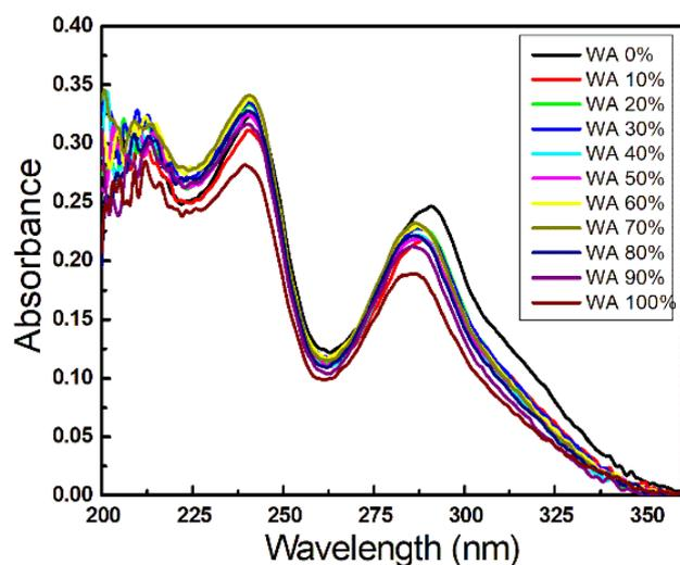
**Figure S1.** Absorption spectra of EBINP in mixed solvent systems (Concentration of EBINP is 8.49  $\mu\text{M}$ )
