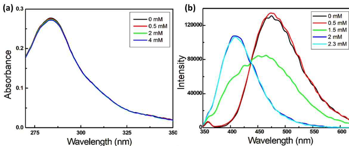
**Figure S4.** (a) absorption spectra and (b) emission spectra ( $\lambda_{\text{exc}}$  320 nm) of EBINP in gradual addition of NaOH (0.25 M) in water medium.
