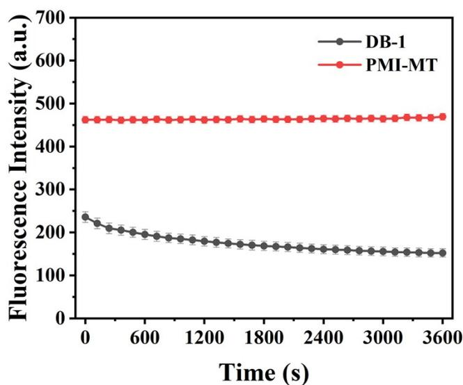
**Fig. S8.** The photostability of the probe **PMI-MT** ( $10 \mu\text{M}$ ) and **DB-1** ( $10 \mu\text{M}$ ) with continuous laser
