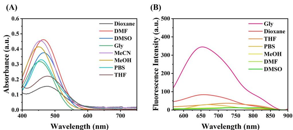
**Fig. S6.** (A) Absorption spectra of the probe **DB-1** in different solvents. (B) Fluorescence intensity spectra of the probe **DB-1** in different solvents.  $\lambda_{\text{ex}} = 470 \text{ nm}$ , slit width:  $d_{\text{ex}} = d_{\text{em}} = 5 \text{ nm}$ .
