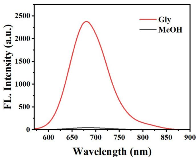
**Fig. S5.** Spectral properties of the probes **PMI-MT** in various solvents. (MeOH and Gly).
