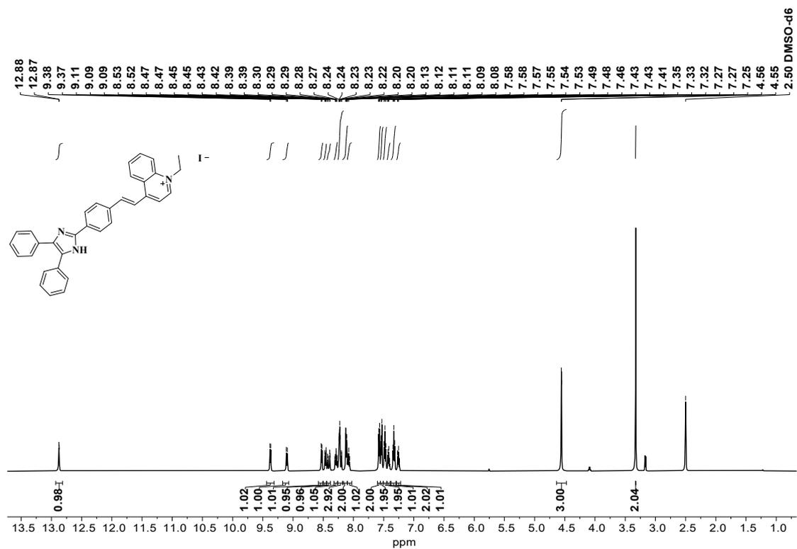
Fig. S21. The  $^1\text{H}$  NMR spectrum of the compound **DB-1** in DMSO.
