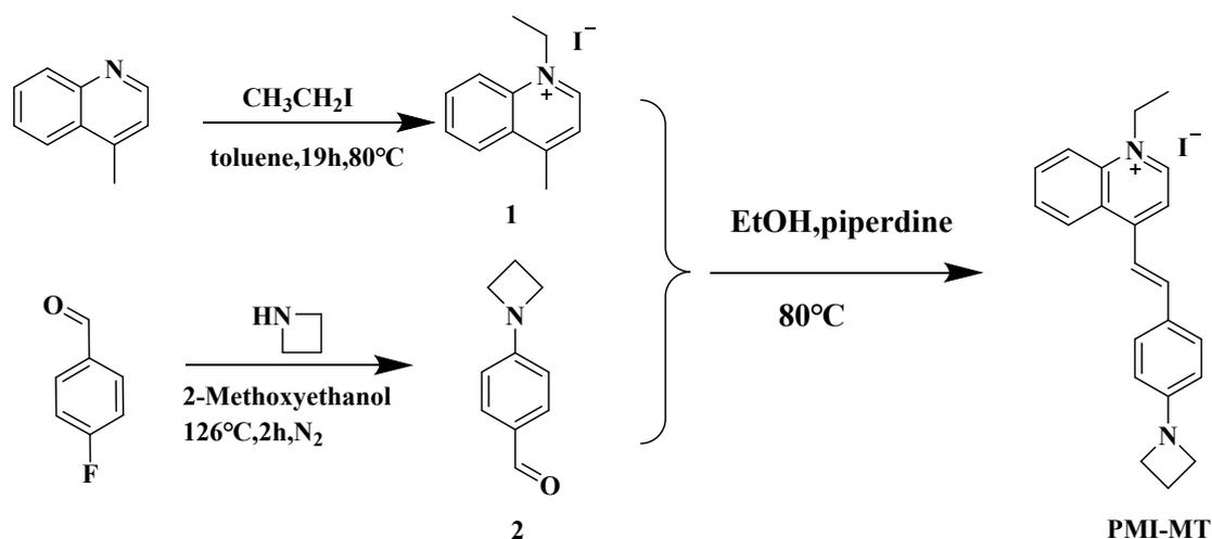
Fig. S1 Steps in the synthesis of the compound PMI-MT
