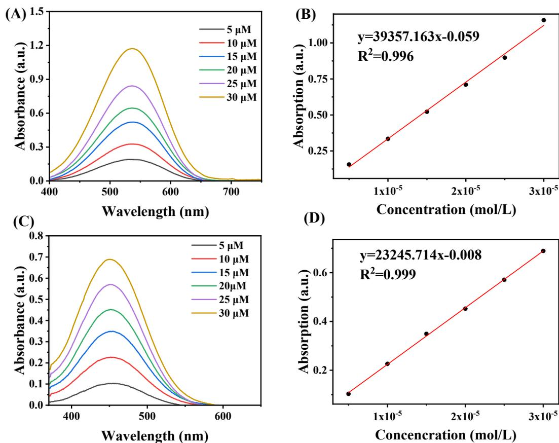
**Fig. S9.** (A) Absorption spectra of different concentrations of probe **PMI-MT** in methanol. (B) Linearity of different concentrations of probe **PMI-MT** with their absorbance in methanol. (C) Absorption spectra of different concentrations of probe **DB-1** in methanol. (D) Linearity of different concentrations of probe **DB-1** with their absorbance in methanol.
