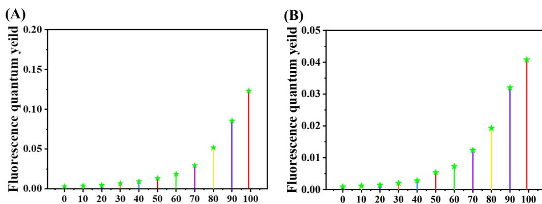
**Fig. S10.** (A) Fluorescence quantum yield ( $\Phi_f$ ) of **PMI-MT** in the Glycerol /MeOH (v/v) mixture. (B) Fluorescence quantum yield ( $\Phi_f$ ) of **DB-1** in the Glycerol /MeOH (v/v) mixture.
