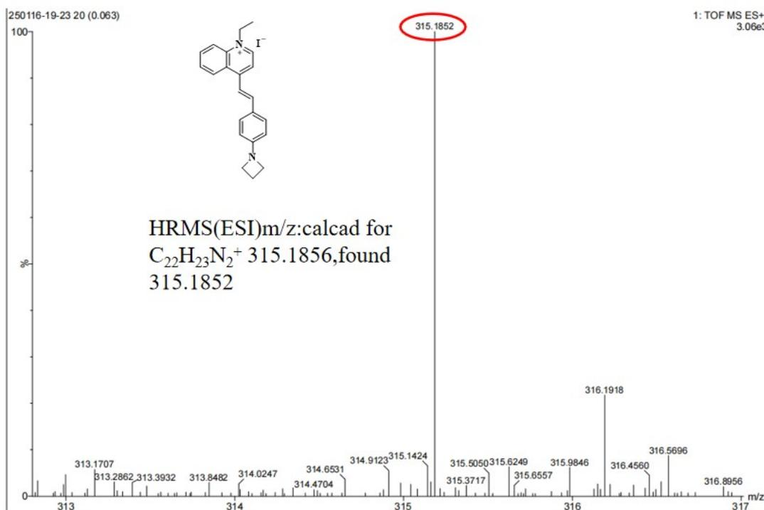
Fig. S20. The HRMS spectrum of the probe **PMI-MT**.
