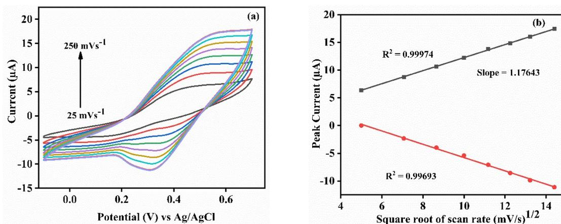
Fig.S1. (a) CV curves obtained at different scan rates for 10%  $\alpha$ -Ni(OH)<sub>2</sub>@DEHP/ CPE using 5 mM redox in 0.1 M KCl. (b) Plot of peak current  $I_p$  [A] vs. square root of scan rate [ $\text{u}^{1/2} (\text{mV s}^{-1})^{1/2}$ ].
