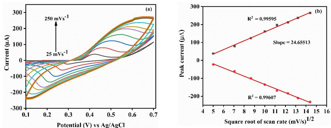
Fig. S2 (a) CV curves at different scan rates from 25 mV s<sup>-1</sup> to 250 mV s<sup>-1</sup> at 10% α-Ni(OH)<sub>2</sub>@DEHPA/CPE using 3 mM glucose in 1 M NaOH. (b) The plot of peak current I<sub>p</sub> [μA] vs square root of scan rate [ν<sup>1/2</sup>(mV s<sup>-1</sup>)<sup>1/2</sup>] in the range of 25 mV s<sup>-1</sup> to 250 mV s<sup>-1</sup>.
