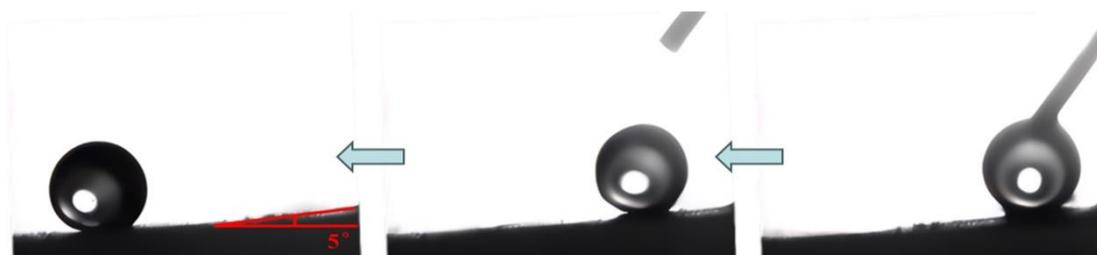
**Figure S7** SPU-66 Rolling angle test.
